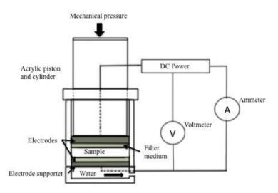
For the design of electro osmotic dewatering of flax, treatment time is one of the most important factors to be considered and it is to be derived in terms of initial and final solid concentrations [41]. In an electro-osmotic cell, the volume of the sample in the cell V, is expressed as the product of cross sectional area of the cell and the thickness of the sample:
