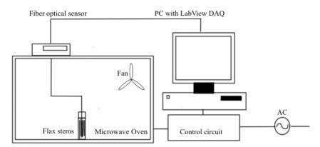
Figure 1. Schematic diagram of a microwave treatment system [28].
