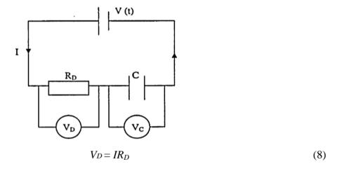
When the power supply switched on, the initial voltage  $V_0$  is independent of the capacitor C. Thus,
