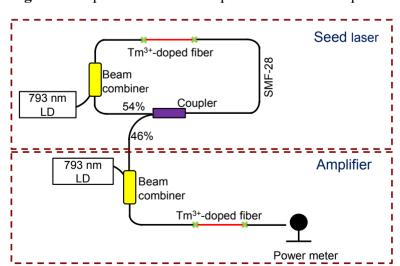
Figure 5. Experimental Tm<sup>3+</sup>-doped silicate fiber amplifier.
