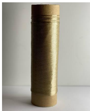
Figure 10. Photograph of a filament bobbin made from 7% solutions of flax noils cellulose in NMMO.
