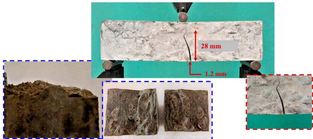
**Figure 17.** CFs concentration at the rupture interface in the case of CFs' dry mixing method.
