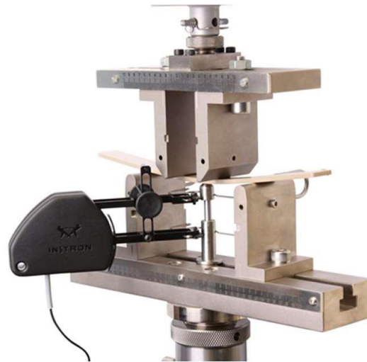
Figure 8. Flexure testing ASTM D790 [22] (Image courtesy of Instron).
