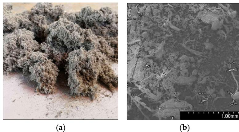
**Figure 1.** Deink paper sludge: (a) sample of cellulose fibers milled with a hammer mill and (b) SEM analysis.
