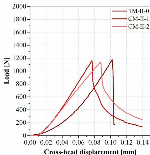
**Figure 6.** Load vs. cross-head displacement curves for representative flexural mortar specimens.
