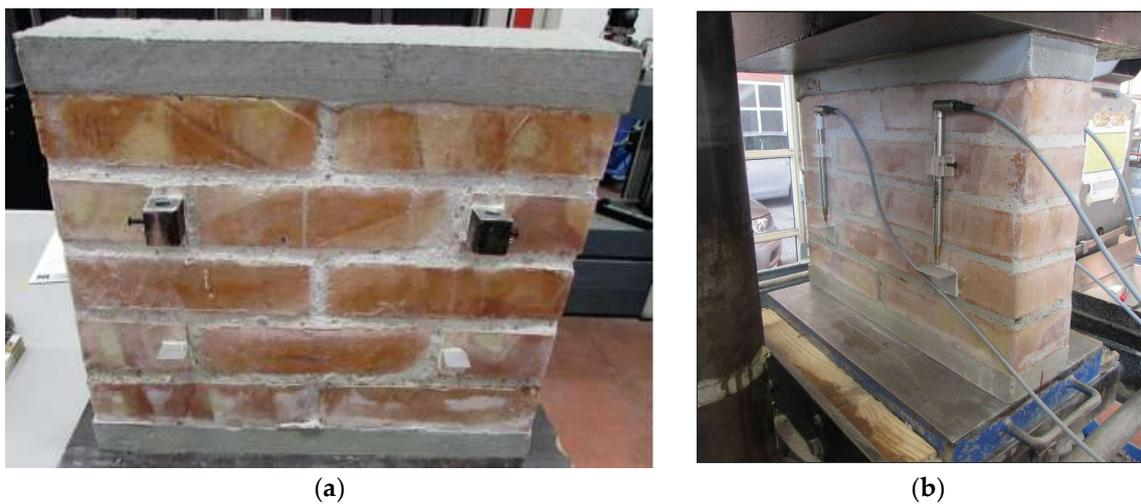
**Figure 5.** Compression test: (a) masonry wall specimen and (b) overview of the test set-up.
