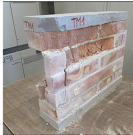
**Figure 9.** Typical failure mode observed in the compression tests on masonry walls (example of failure mode observed in specimen MW-TM-1).
