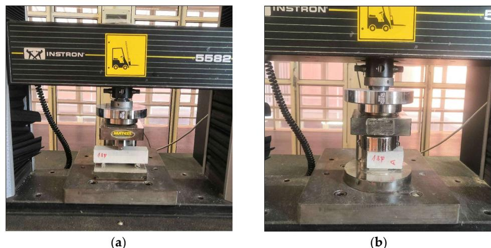
**Figure 3.** Mechanical characterization tests: (a) flexural and (b) compression test set-up.
