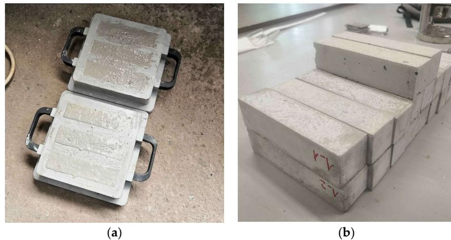
**Figure 2.** Cement-based mortar preparation: specimens in (a) fresh and (b) hardened state.
