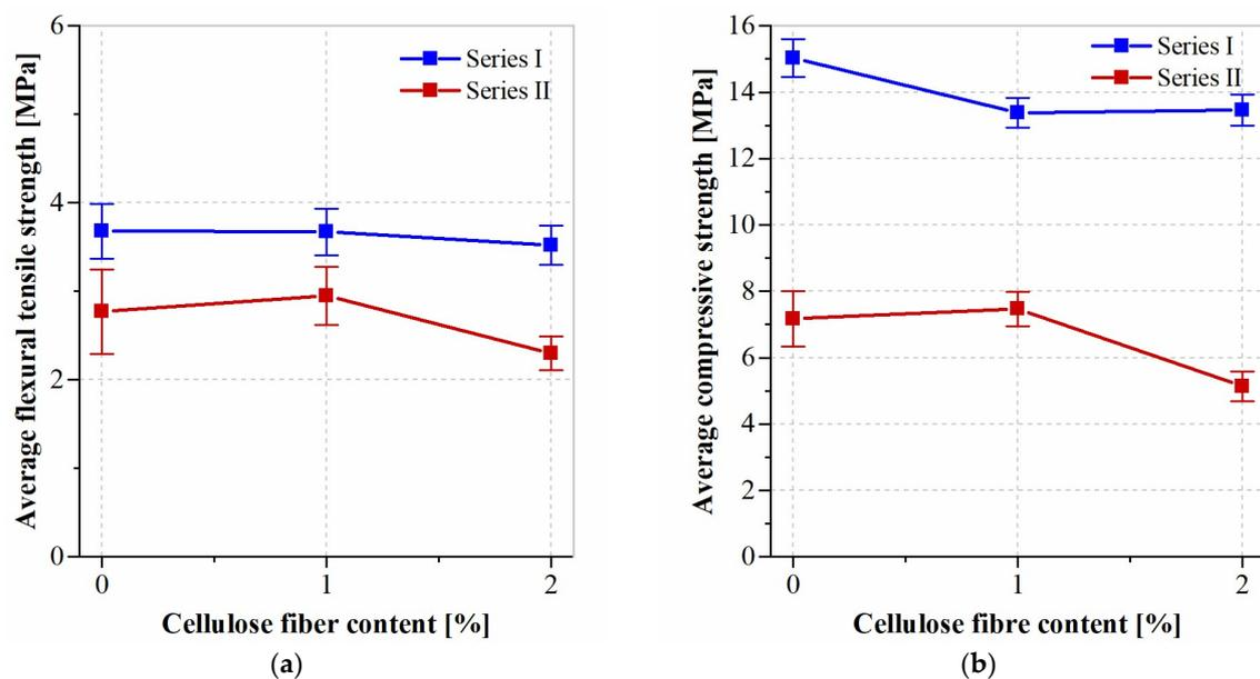
**Figure 7.** Mechanical property variations of the mortar with cellulose fiber content: (a) average flexural tensile strength and (b) compressive strength.
