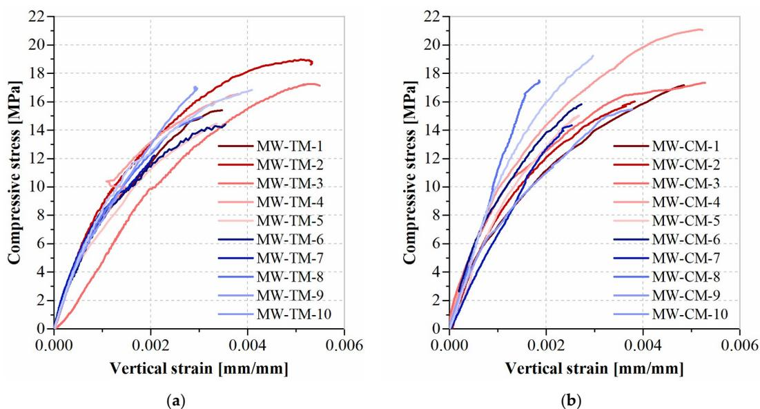
**Figure 8.** Compressive stress vs. vertical strain curves of masonry walls made with (a) traditional and (b) eco-friendly mortars.
