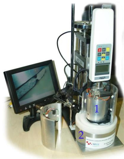
**Figure 2.** Multi-purpose differential conductometer: 1-measuring cylinder, 2-measuring base.
