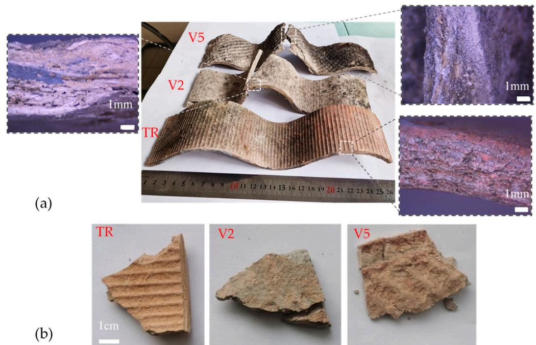
**Figure 1.** The primary appearance of tested samples and optical microscope view of the widths (a); the view of pieces of samples after thermal treatment at 1100 °C (b).
