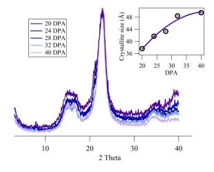
**Figure 4.** XRD spectra of cotton fibers harvested at different developmental time points; 20, 24, 28, 32 and 40 DPA. Inset figure shows the cellulose crystallite size as calculated by the Scherrer equation.
