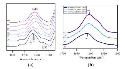
**Figure 3.** (a) FTIR spectra of the O-H bending region for cotton fibers harvested at different DPA: (a) 18 DPA; (b) 20 DPA; (c) 24 DPA; (d) 28 DPA; (e) 32 DPA; (f) 36 DPA; and (g) 40 DPA; (b) O-H bending region (deuterated) harvested at 18 DPA (bottom), 24 DPA (middle), and 40 DPA (top).
