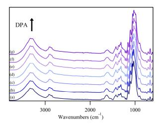
**Figure 1.** FTIR spectra of cotton fibers harvested at different DPA: (a) 18 days post-anthesis (DPA); (b) 20 DPA; (c) 24 DPA; (d) 28 DPA; (e) 32 DPA; (f) 36 DPA; and (g) 40 DPA. Spectra are shown shifted along the y-axis.
