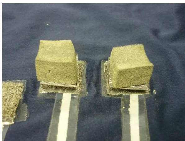
Figure 8. Conductive foam blocks on the smart shirt.
