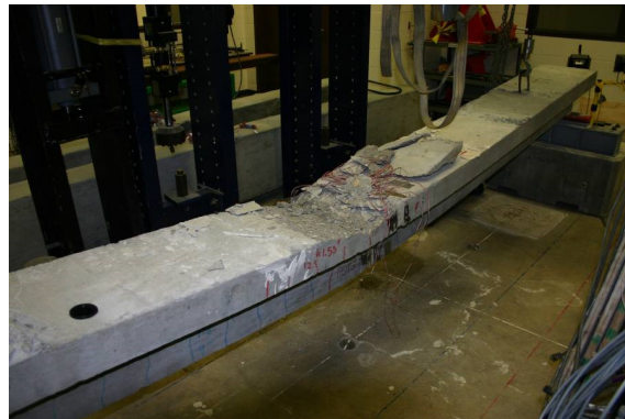
Figure 3. Beam T1 at failure.
