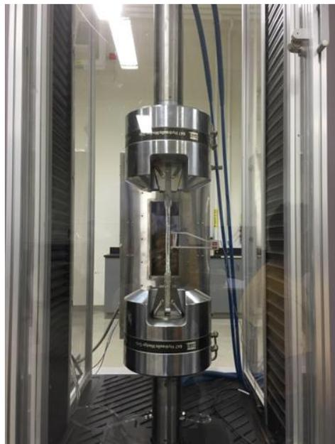
**Figure 3.** Clamping grips.
