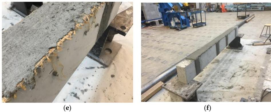
**Figure 7.** Strengthening procedure: (a) initial mortar layer applied; (b) FRCM mesh partially embedded inside the mortar; (c) FRCM mesh embedded totally inside the mortar; (d) U-wrapped FRCM strips embedded inside the mortar; (e) FRCM mesh covered with mortar; (f) finishing after the application of the second FRCM layer.
