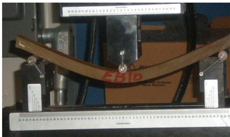
**Figure 4.** Large deflection of the epoxy beam (EB10) after 40 Cycles at 100 °C.
