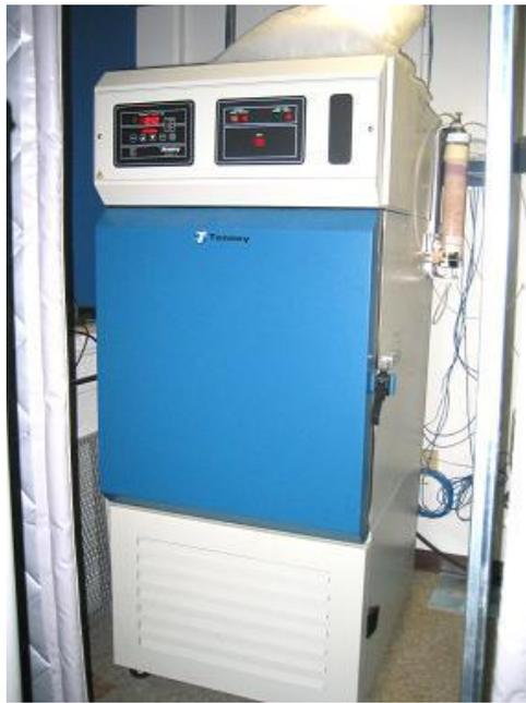
**Figure 1.** Environmental chamber (model: Tenny T10RC-1.5 SPL) (Tenny Engineering, 1090 SPRINGFIELD RD, Union, NJ 07083, United States).
