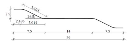
Figure A1. Geometry of the fibers of the case study (dimensions in mm).
