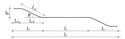
**Figure 1.** Typical geometry of a hooked fiber bar of diameter  $d_f$ . Dimensions and properties of the fiber used for the case study are shown in Appendix A.
