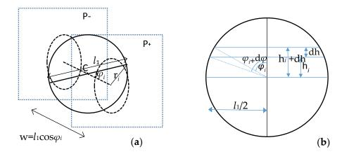
**Figure 7.** Figure for the quantification of factor  $\alpha_{\varphi i}$ : (a) Maximum crack width (w) of the strip that includes the center point of all fibers with orientation angle  $\varphi$  to the plane of the crack (P) that cross it; (b) Ratio of the surface areas of a spherical segment.
