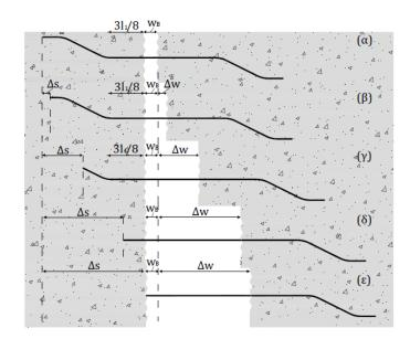
**Figure 3.** Phases  $[(\alpha)-(\varepsilon)]$  of extraction for a fiber, embedded in concrete, due to formation of a perpendicular crack (initial w<sub>B</sub> +  $\Delta$ w). Extraction length ( $\Delta$ s) increases until fiber is fully extracted.
