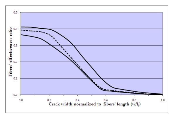
**Figure 10.** The effectiveness ratio of the fiber in relevance with crack width for several steel hooked fibers. (Continuous lines for upper and lower bounds, dotted line for the case study presented in detail).
