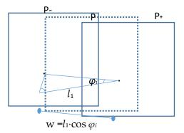
**Figure 6.** Width (w) of strip that includes the center point of all fibers with orientation angle  $\varphi$  to the plane of the crack (P) that they cross.
