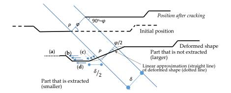
**Figure 4.** Modeled deformation of a single fiber crossing a crack ( $\varphi$  is the inclination of the fiber from the perpendicular to the crack direction, and  $\delta$  is the width of the crack). (**a**)shortening of the smaller part of the fiber due to extraction; (**b**) reaction stresses of concrete against compression and (**c**) against bending, and (**d**) friction stresses along the deformed fiber axis, due to (**b**) and (**c**).
