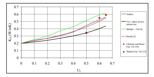
Figure 11. Theoretical values of transverse thermal conductivity versus filler content.
