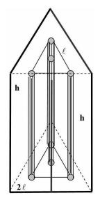
Figure 2. Triangular prismatic representative volume element (RVE).
