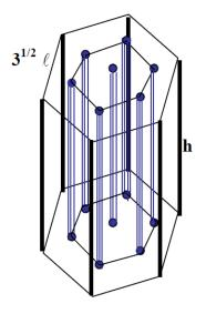
Figure 7. Hexagonal prismatic RVE.
