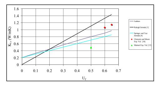
Figure 10. Theoretical values of longitudinal thermal conductivity versus filler content.
