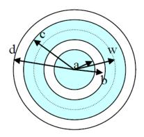
Figure 3. Four-phase coaxial cylindrical model.
