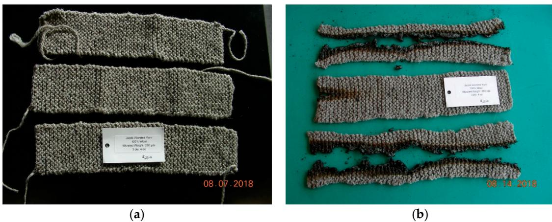
Figure 15. Jacob Wool Vertical Burn—before testing (a) and after testing (b).
