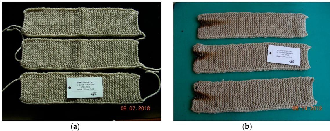
**Figure 16.** CVM/Romeldale Blend Vertical Burn—before testing (a) and after testing (b).
