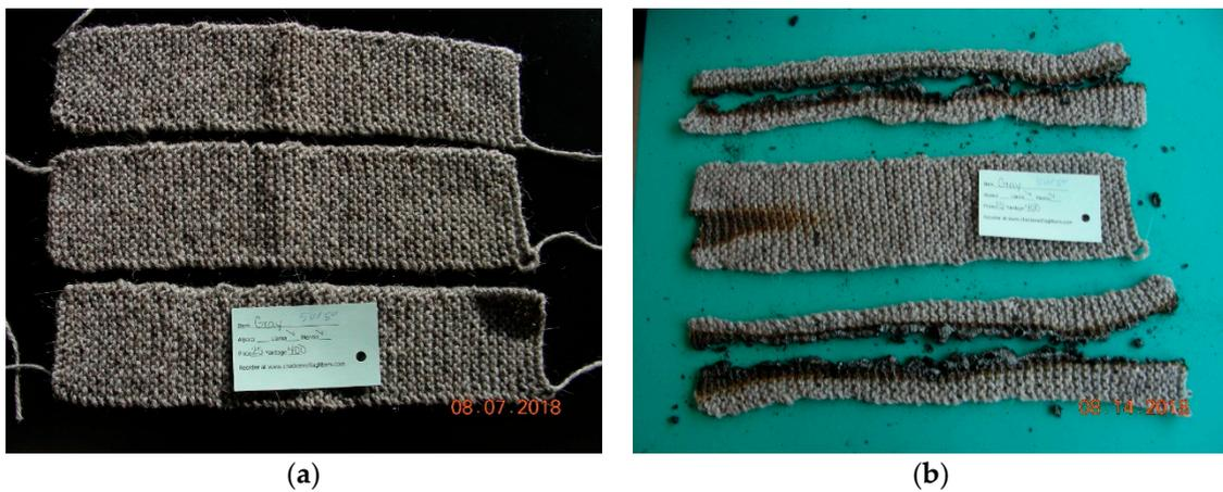
Figure 14. Llama/Merino Blend Vertical Burn—before testing (a) and after testing (b).
