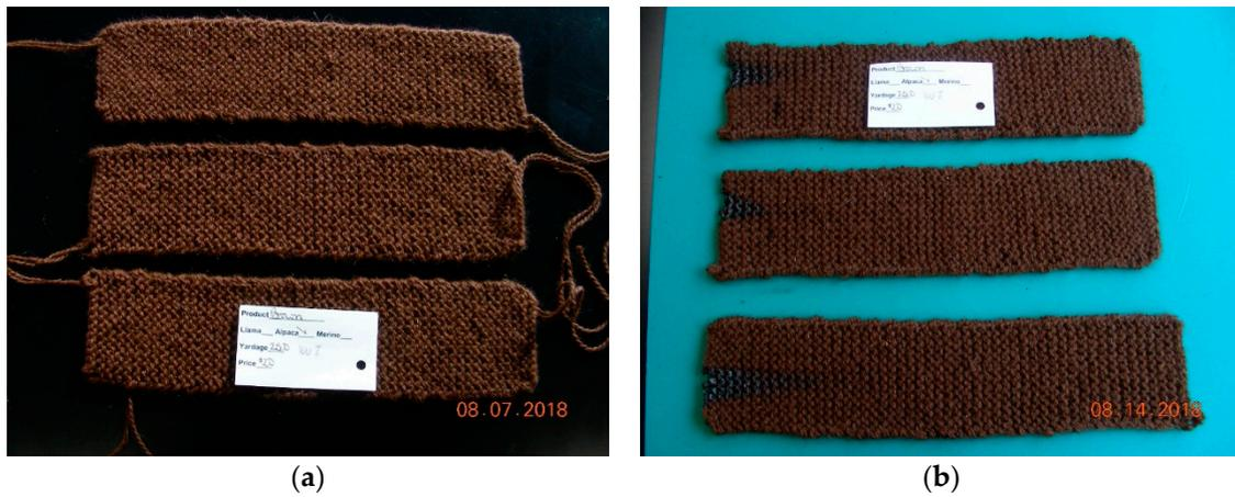
Figure 13. Brown 100% Alpaca Vertical Burn—before testing (a) and after testing (b).
