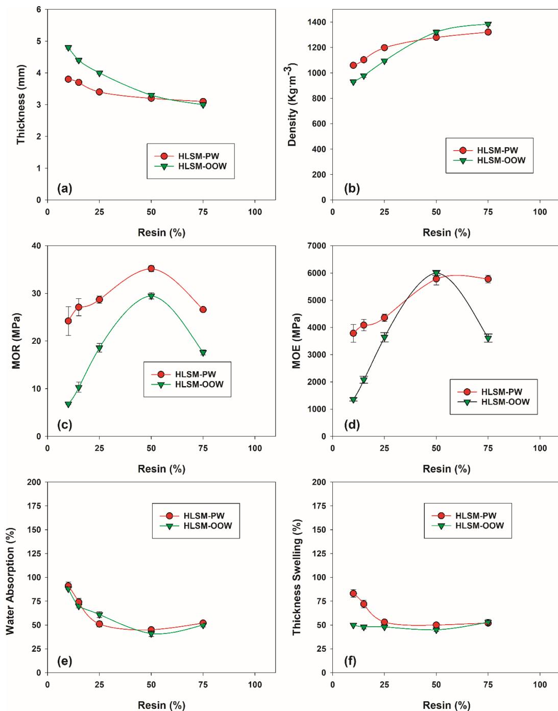
**Figure 6.** The influence of HLSM on the dimensional, flexural and dimensional stability properties of various CWP. Curve plots: (a) Thickness, (b) density, (c) MOR, (d) MOE, (e) water absorption, (f) thickness swelling.
