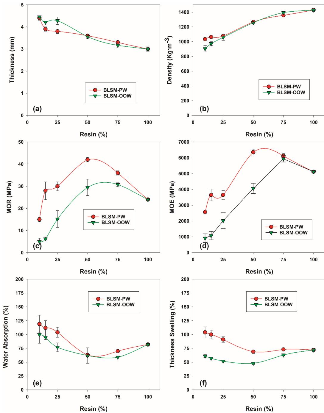
**Figure 5.** The influence of BLSM on the dimensional, flexural and dimensional stability properties of various CWPs. Curve plots: (a) Thickness, (b) density, (c) MOR, (d) MOE, (e) water absorption, (f) thickness swelling.
