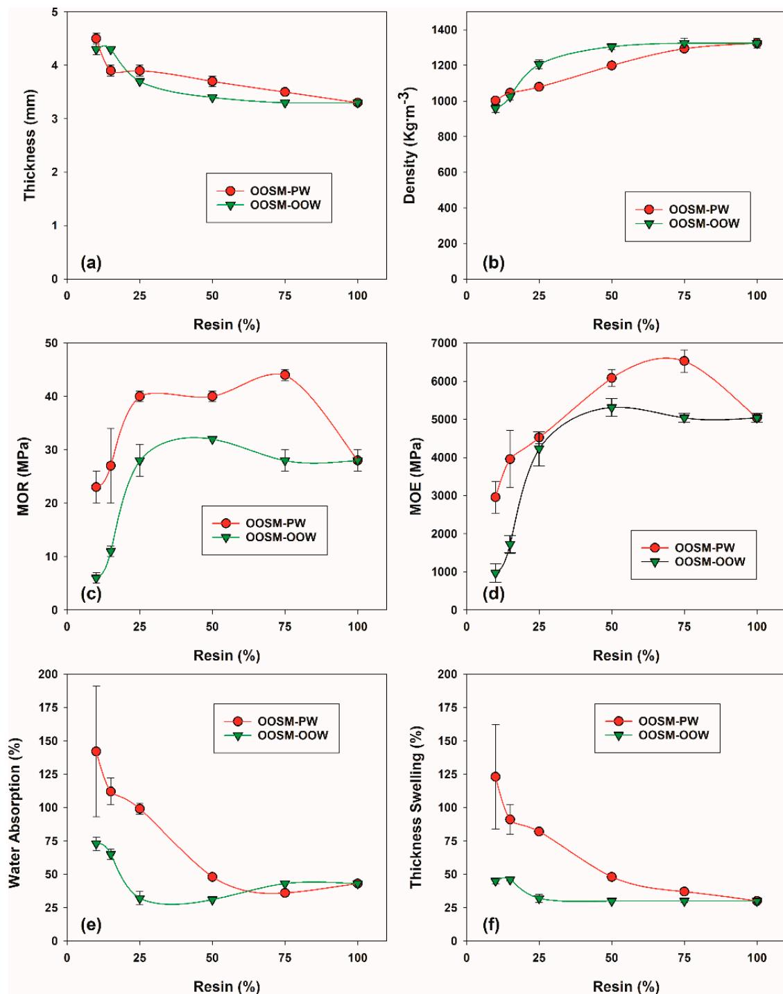
**Figure 4.** The influence of OOSM on the dimensional, flexural and dimensional stability properties of various CWP. Curve plots: (a) Thickness, (b) density, (c) MOR, (d) MOE, (e) water absorption, (f) thickness swelling.
