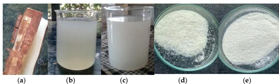
**Figure 1.** (a) Untreated CP, (b) CNF procedure I colloid, (c) CNF procedure II colloid, (d) CNF procedure I powder, and (e) CNF procedure II powder.
