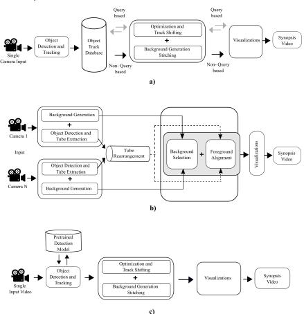
**Figure 3.** An illustration of different synopsis methodologies and their components: (a) single-camera video synopsis framework; (b) multi-camera video synopsis framework; (c) abnormal content video synopsis framework.
