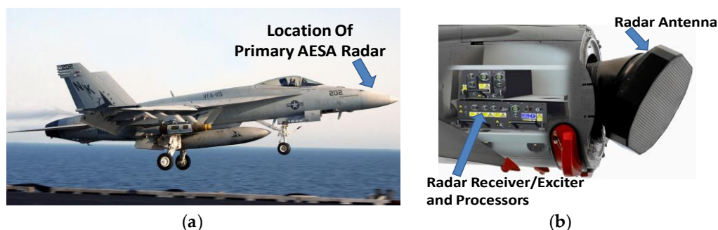
Figure 2. Active Electronically Scanned Arrays (AESAs) are used on (a) F/A-18E/F Super Hornet with an AESA phased array located in the nose of the aircraft; and (b) Euroradar CAPTOR mounted onto the nose of a Eurofighter Typhoon aircraft.
