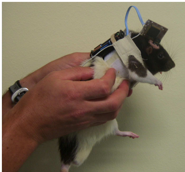
Figure 20. Arrangement for in vivo measurements. Note the headstage, the battery backpack and the whip antenna placed along the back of the animal.
