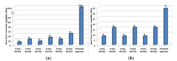
Figure 6. Burst error (a) detection capability; and (b) correction capability (1024-bit cache line).
