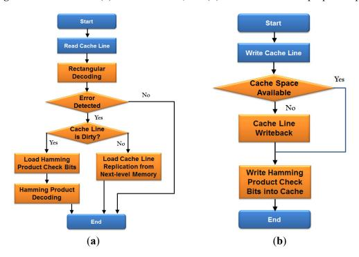
Figure 3. Flow chart of (a) Cache line read, and (b) Cache line write of proposed approach.
