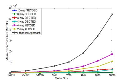
**Figure 9.** METF comparison (cache line size = 512 bits).
