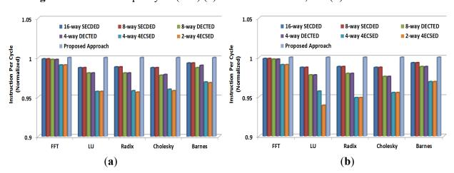
**Figure 12.** Instruction per cycle (IPC) (a) 1024-bit cache line, and (b) 512-bit cache line.
