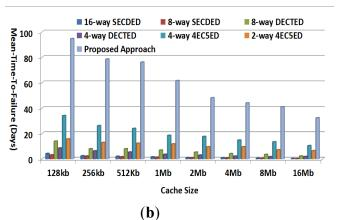
**Figure 11.** METF comparison (a) Cache line size = 512 bits, fault rate  $10^{-5}$ /day, and (b) Cache line size = 512 bits, fault rate  $10^{-4}$ /day.
