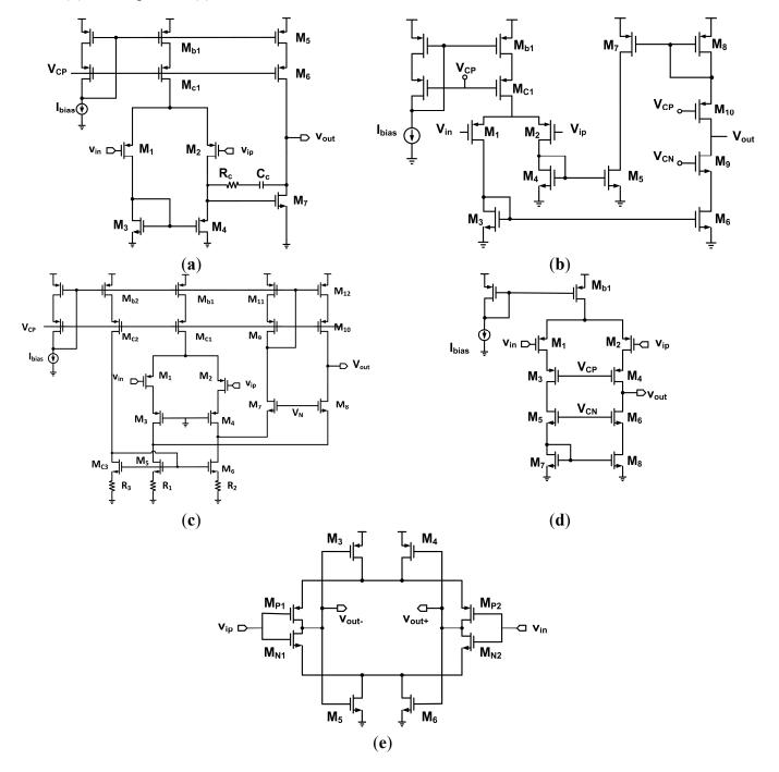
The previously mentioned topologies can be implemented in differential form. In [21], several differential architectures including closed-loop fully differential, telescopic-cascode amplifier;
