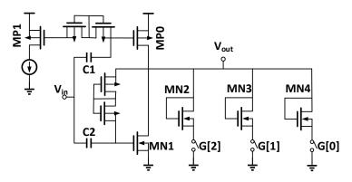
Figure 6. Classic neural amplifier topology with capacitive feedback.
