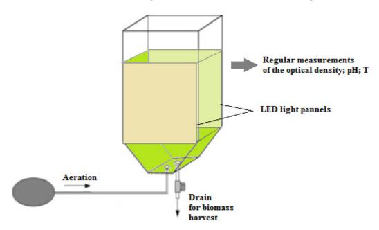
Figure 1. Scheme of the 100-L photobioreactor for microalgae cultivation.
