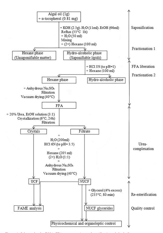
Figure 2. Scheme for the DHA-EPA concentration and purification of algal oil.
