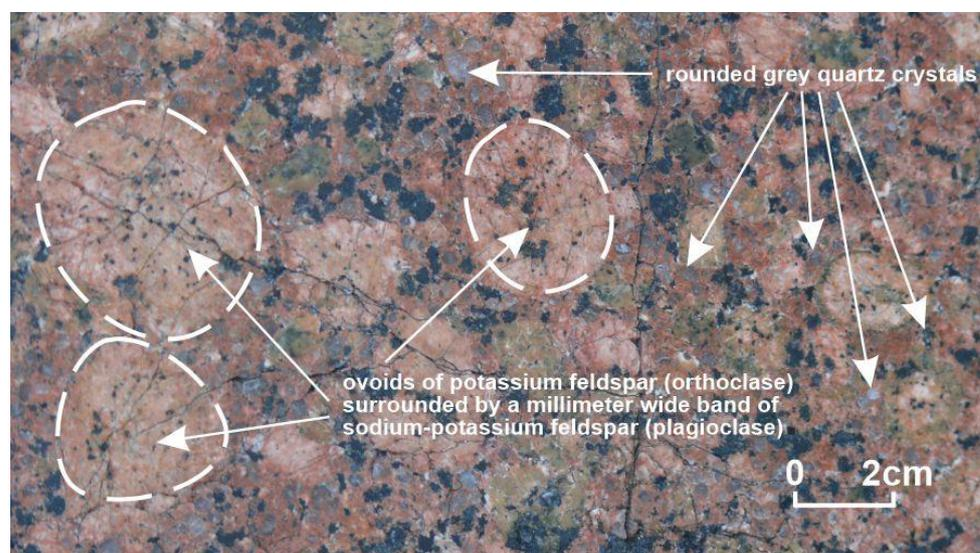
**Figure 25.** Details of the structure and texture of the Åland rapakivi granite.
