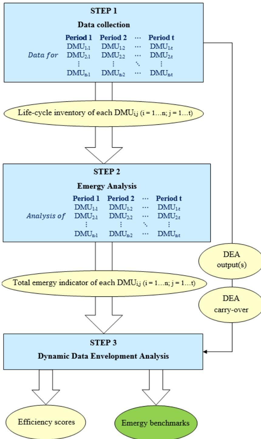
Figure 1. Representation of the Em + DynDEA method.
