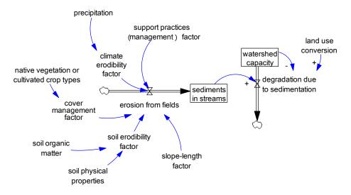
**Figure 6.** Soil erosion model based on the RUSLE framework used to simulate erosion dynamics at the field scale, based on local soil, climate, and management practices, with land use change in the watershed. Adapted and simplified from [94].
