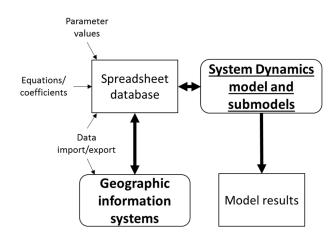
**Figure 7.** Conceptual diagram displaying the interface capabilities of SD with other programs used in land use and soil erosion analyses; modified from [96].
