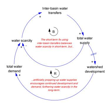
**Figure 4.** "Fixes that backfire" archetype identified by [65]. The "quick fix" of delivering inter-basin transfers alleviates (or balances) water scarcity in the short-term, but makes it worse in the long-term by encouraging (or reinforcing) watershed development. Adapted and expanded based on [65].
