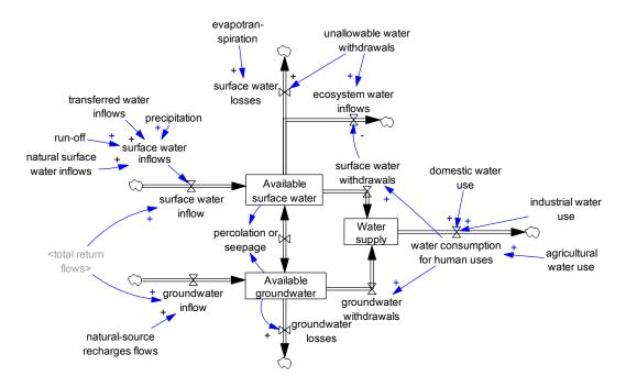
**Figure 3.** Hydrology sub-system similarly adapted and simplified from [65], displaying natural and anthropogenic-driven water flows, including domestic, industrial, and agricultural water demand that drives inter-basin transfers from surface water, further developing the watershed and ultimately total water demand.
