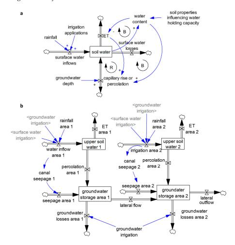
**Figure 5.** Soil water model used to simulate (**a**) soil water in the surface layer used for estimating soil-water (irrigation)-plant interactions; and (**b**) the surface water-groundwater interactions driven by irrigation applications and groundwater abstraction between fields. Adapted and simplified from [90].
