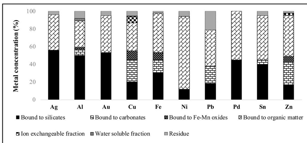
**Figure 4.** Sequential extraction of metals using various extraction reagents ( $n = 3$ ).
