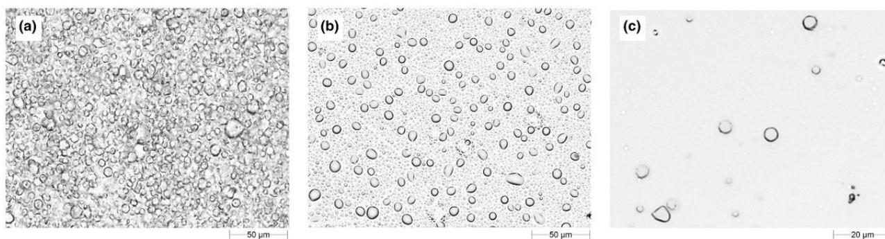
**Figure 8.** Optical microscopy of an emulsion based on silicone emulsions at different dilutions from (a) concentrated, (b) 50/50 vol./vol., to (c) diluted.
