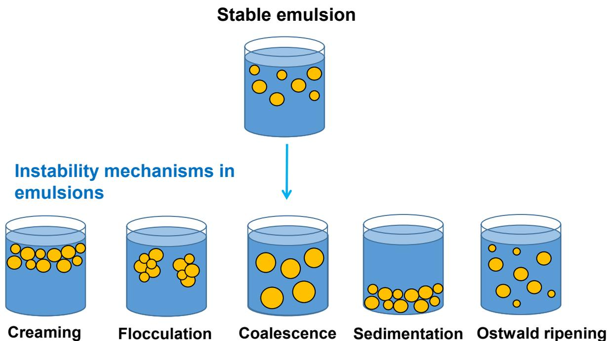
**Figure 7.** Schematic of dispersion instability phenomena: creaming, flocculation, coalescence, sedimentation, and Ostwald ripening. Adapted from [117].
