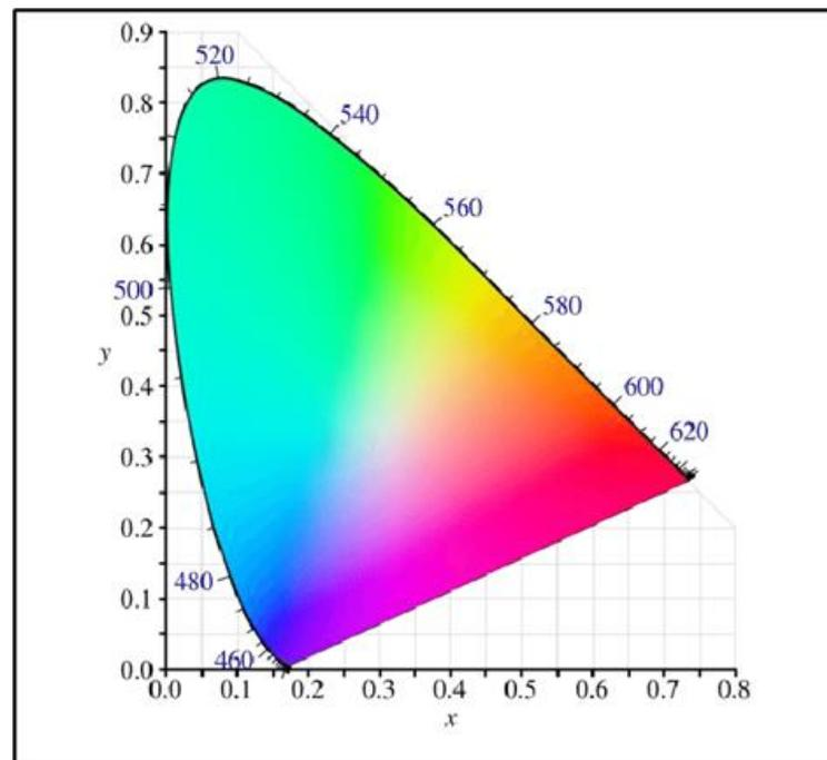
**Figure 17.** CIE 1931 color space. Y signifies luminance; Z is roughly equal to the blue stimulus (S cones), and X is a mix tending toward the red-to-green sensitivity curve [210].
