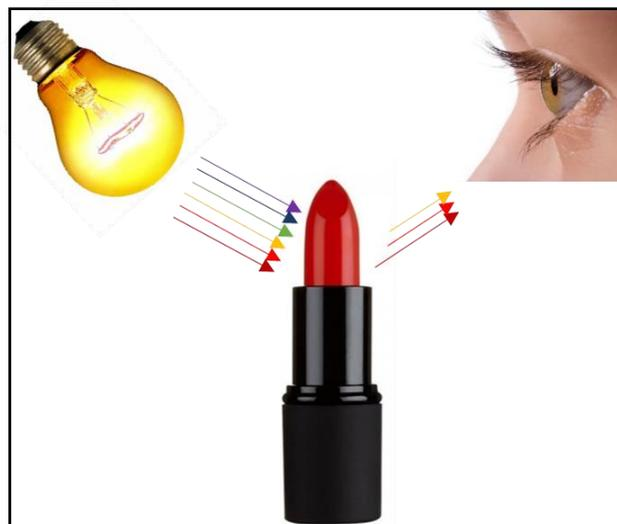
**Figure 15.** Elements for color perception: a light source illuminating an object, the object reflecting or transmitting light to an observer, and the observer perceiving the reflected light.
