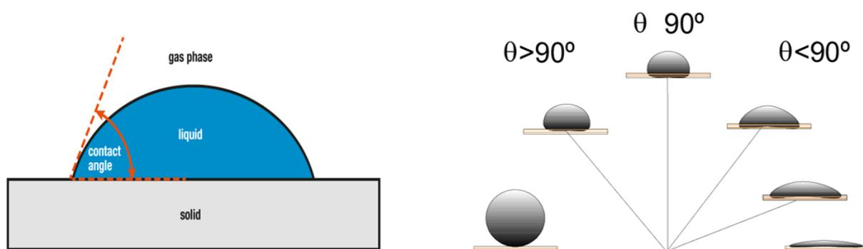
**Figure 12.** Contact angles less than 90 degrees indicate that the droplet wets the surface. A contact angle of 90 degrees signifies that the cohesion and adhesion forces are equal, typically observed when a solid particle exhibits mixed wettability between oil and water. Contact angles greater than 90 degrees imply that the droplet does not wet the surface.
