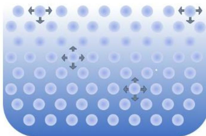
**Figure 11.** Forces associated with interfacial tension.
