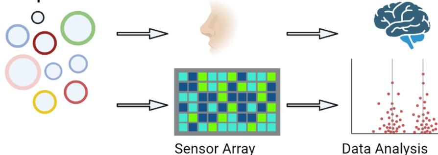
**Figure 6.** Comparison of the biological olfactory system and the electronic nose. The sensor array acts as an olfactory receptor that detects chemical compounds and emits a signal, which is then processed. (Image created with BioRender.com, accessed on 7 July 2023).
