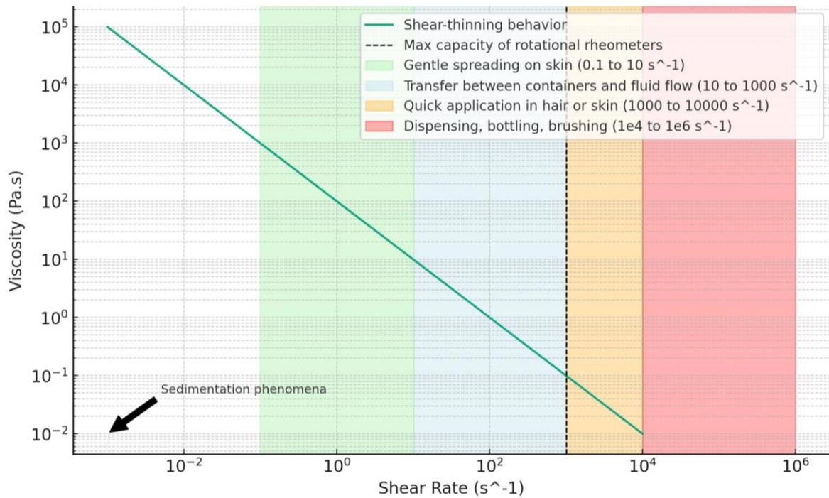
**Figure 13.** Representation of a flow curve for shear-thinning cosmetic products (green line). Cosmetic products are mainly dispersions that present sedimentation phenomena at very low shear rates. Then, higher shear applications such as gentle spreading on the skin, transfer between containers and fluid flow, quick application to hair or skin, and dispensing, bottling, and brushing are represented by very-high shear processes that cannot be measured using conventional rotational rheometers.
