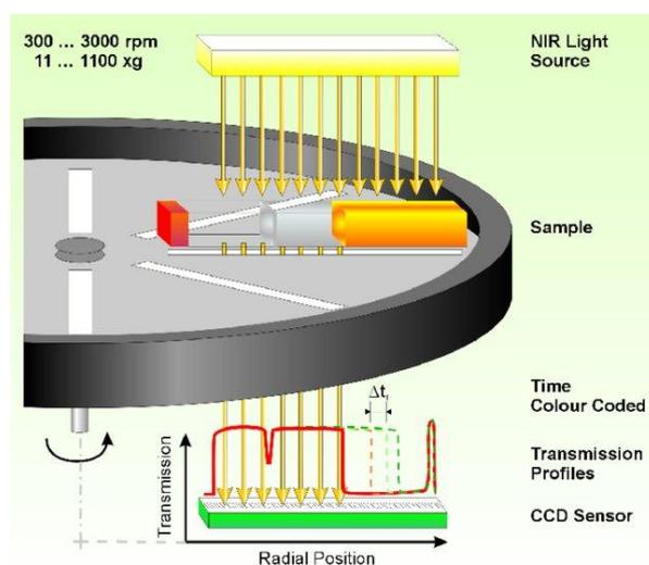
**Figure 9.** General structure for the LUMiSizer. From the *LUMiSizer Manual*.
