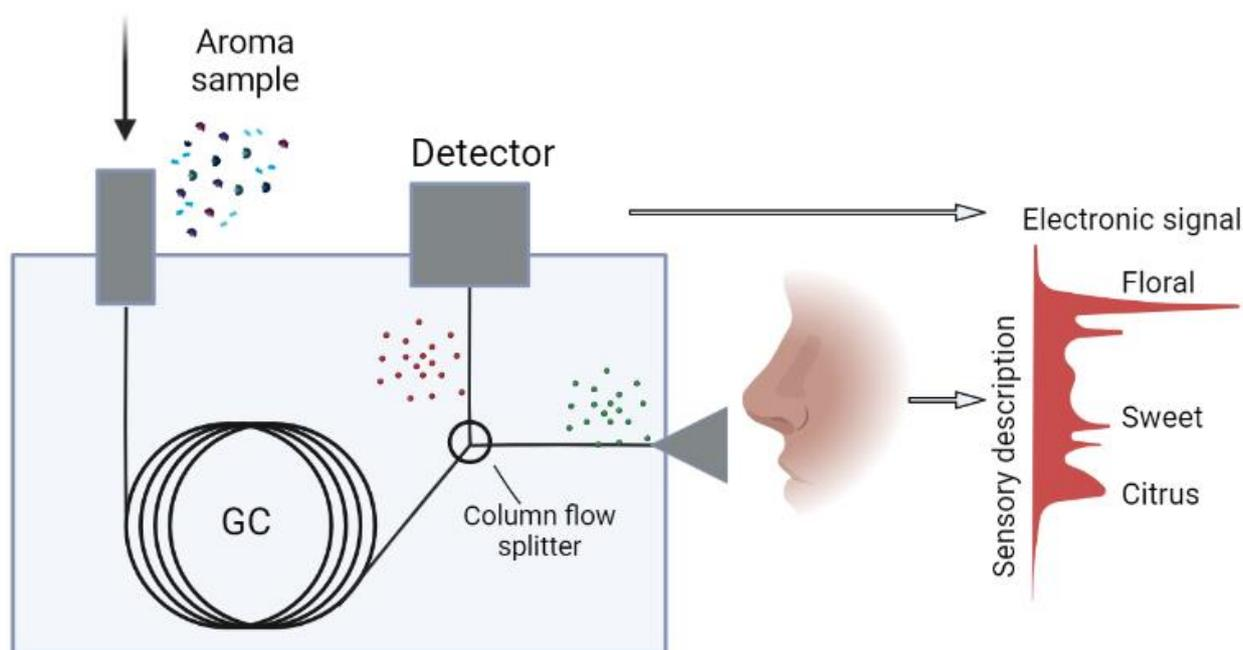
**Figure 4.** Diagram of a gas chromatograph coupled with an olfactometer. This system has a Y splitter (three-way splitter or two-way splitter) that allows the sample to reach one or two instrumental detectors as well as the olfactometer. (Image created with BioRender.com).
