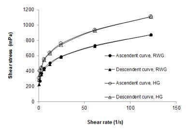
Figure 2. Rheograms of the rice water hydrogel (RWG) and the control hydrogel (HG).
