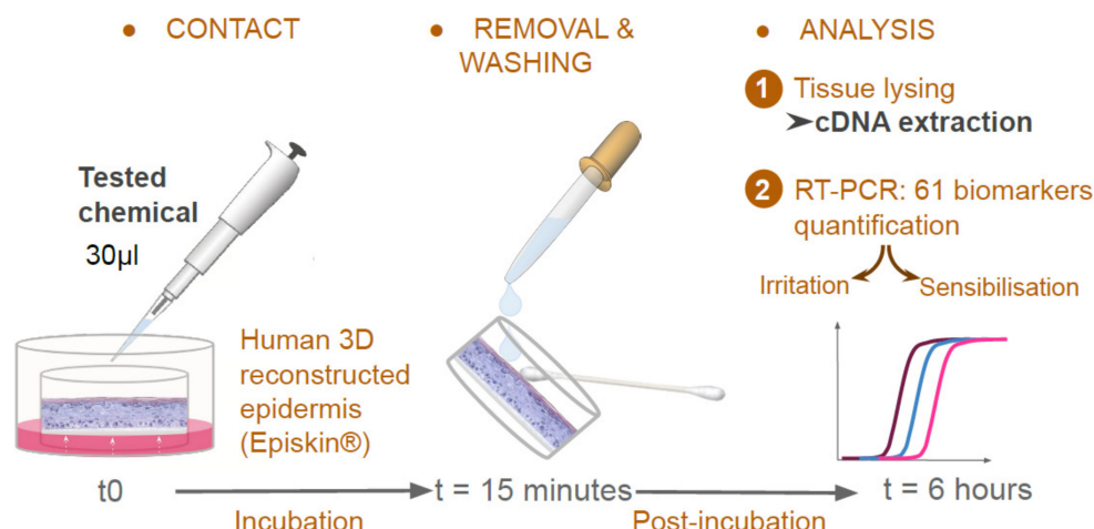
Figure 4. Sens-Is Assay according to Immunosearch Standard Operating Protocol (SOP), analyzing the expression of a panel of genes by RT-PCR in a reconstructed human epidermis model exposed to topical application of a test chemical.
