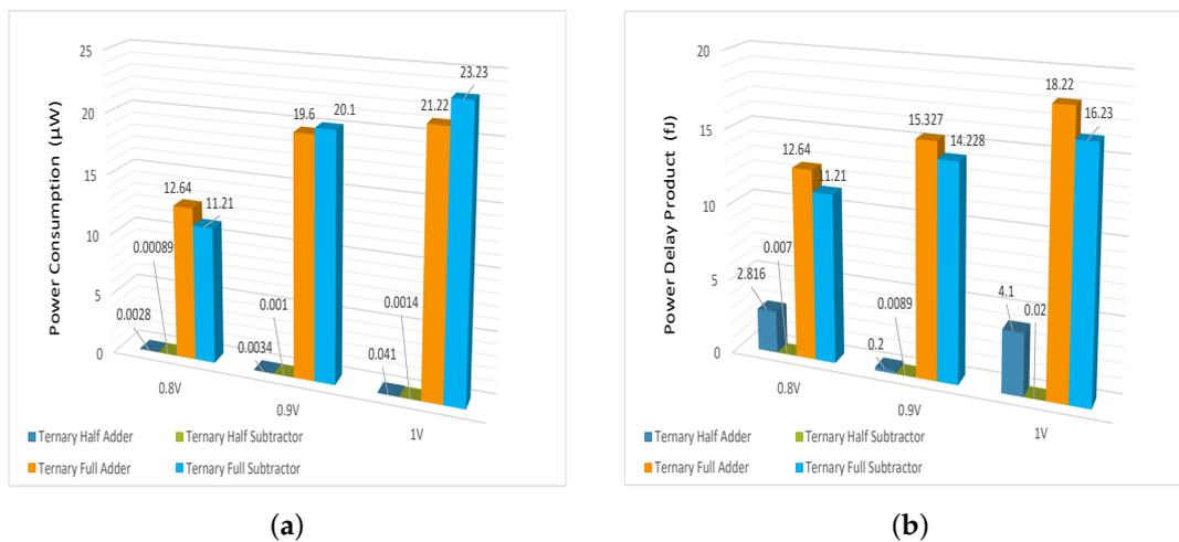
Figure 16. Effect of varying operating voltage on (a) Power Consumption (b) Power Delay Product.
