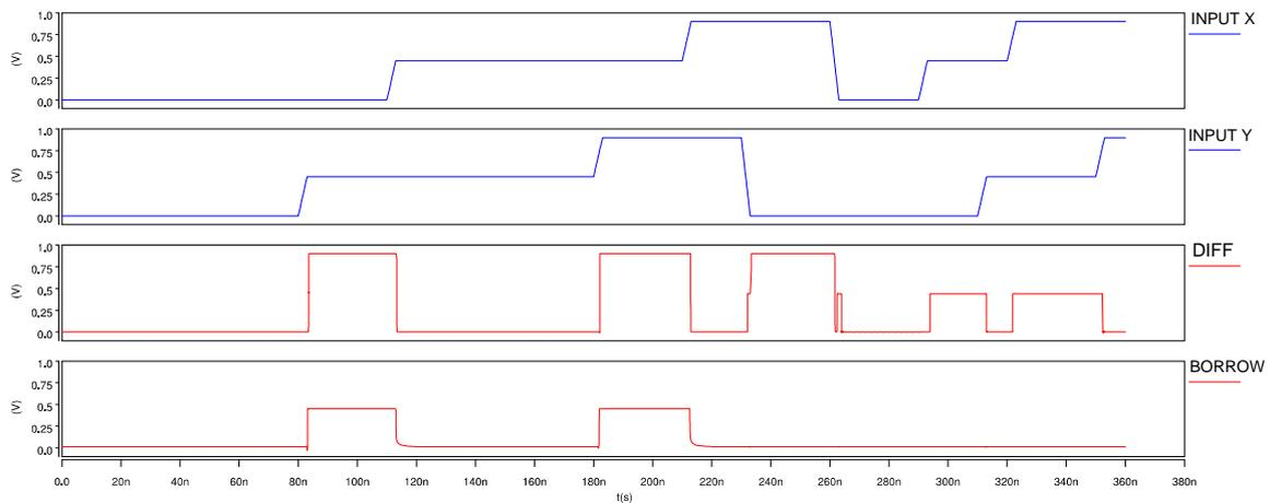
**Figure 12.** Input and Output waveforms of Ternary Half Subtractor.
