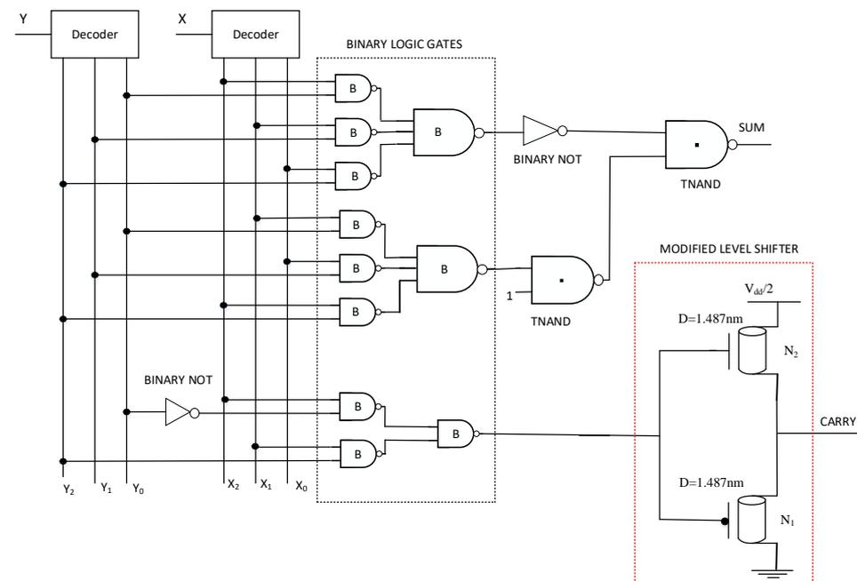
Figure 7. Schematic of Ternary Half Adder.
