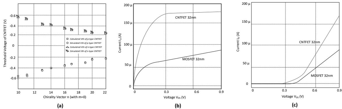
**Figure 2.** (a) CNTFET threshold variation with varying n (for m = 0). (b) Comparison of I-V curve of n-type MOSFET with n-type CNTFET in 32 nm technology for  $I_D$ - $V_{DS}$ . (c) Linear scale  $I_D$ - $V_{GS}$ .
