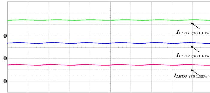
(a) 75% rated power ( $I_{LED1}$ : 200 mA/div,  $I_{LED2}$ : 200 mA/div,  $I_{LED3}$ : 200 mA/div, time: 5 ms/div)
