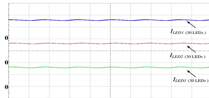
**Figure 9.** Waveforms of  $I_{LED1}$ ,  $I_{LED2}$  and  $I_{LED3}$  with equal number of LEDs. ( $I_{LED1}$ : 200 mA/div,  $I_{LED2}$ : 200 mA/div,  $I_{LED3}$ : 200 mA/div, time: 5 ms/div).
