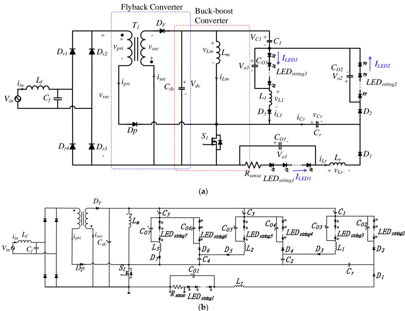
Figure 1. Proposed single-stage single-switch LED drivers (a) three LED strings; (b) seven LED strings.
