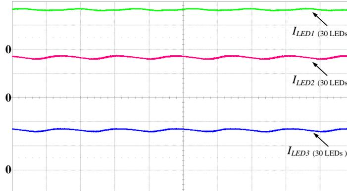
(c) 25% rated power ( $I_{LED1}$ : 100 mA/div,  $I_{LED2}$ : 100 mA/div,  $I_{LED3}$ : 100 mA/div, time: 5 ms/div)
