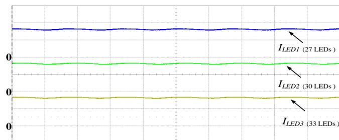
**Figure 10.** Waveforms of  $I_{LED1}$ ,  $I_{LED2}$  and  $I_{LED3}$  with different numbers of LEDs. ( $I_{LED1}$ : 200 mA/div,  $I_{LED2}$ : 200 mA/div,  $I_{LED3}$ : 200 mA/div, time: 5 ms/div).
