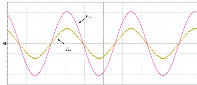
Figure 5. Input voltage and current waveforms. ( $v_{in}$ : 100 V/div,  $i_{in}$ : 1.0 A/div, time: 5 ms/div).
