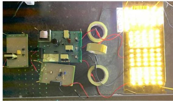
**Figure 14.** 90-W LED prototype circuit.
