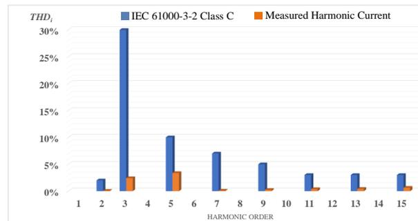
Figure 6. Harmonic spectrum of the input line current.
