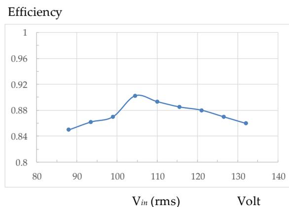
**Figure 11.** Measured circuit efficiency at different input voltages.
