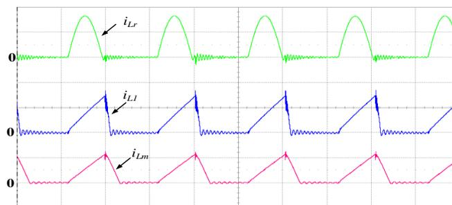
Figure 8. Current waveforms of  $i_{Lr}$ ,  $i_{L1}$  and  $i_{Lm}$ . ( $i_{Lr}$ : 1 A/div,  $i_{Lm}$ : 2 A/div,  $i_{L1}$ : 1 A/div, time: 10  $\mu$ s/div).
