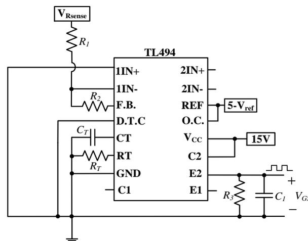
Figure 4. Closed-loop control circuit.
