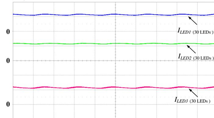
(b) 50% rated power ( $I_{LED1}$ : 200 mA/div,  $I_{LED2}$ : 200 mA/div,  $I_{LED3}$ : 200 mA/div, time: 5 ms/div)
