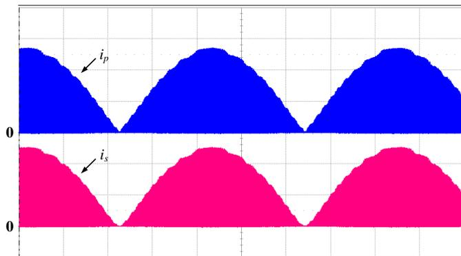
Figure 7. Primary and secondary currents of  $T_1$ . ( $i_p$ : 2 A/div,  $i_s$ : 2 A/div, time: 2 ms/div).
