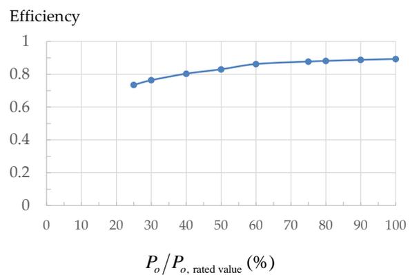
Figure 13. Measured circuit efficiency at different output power levels.
