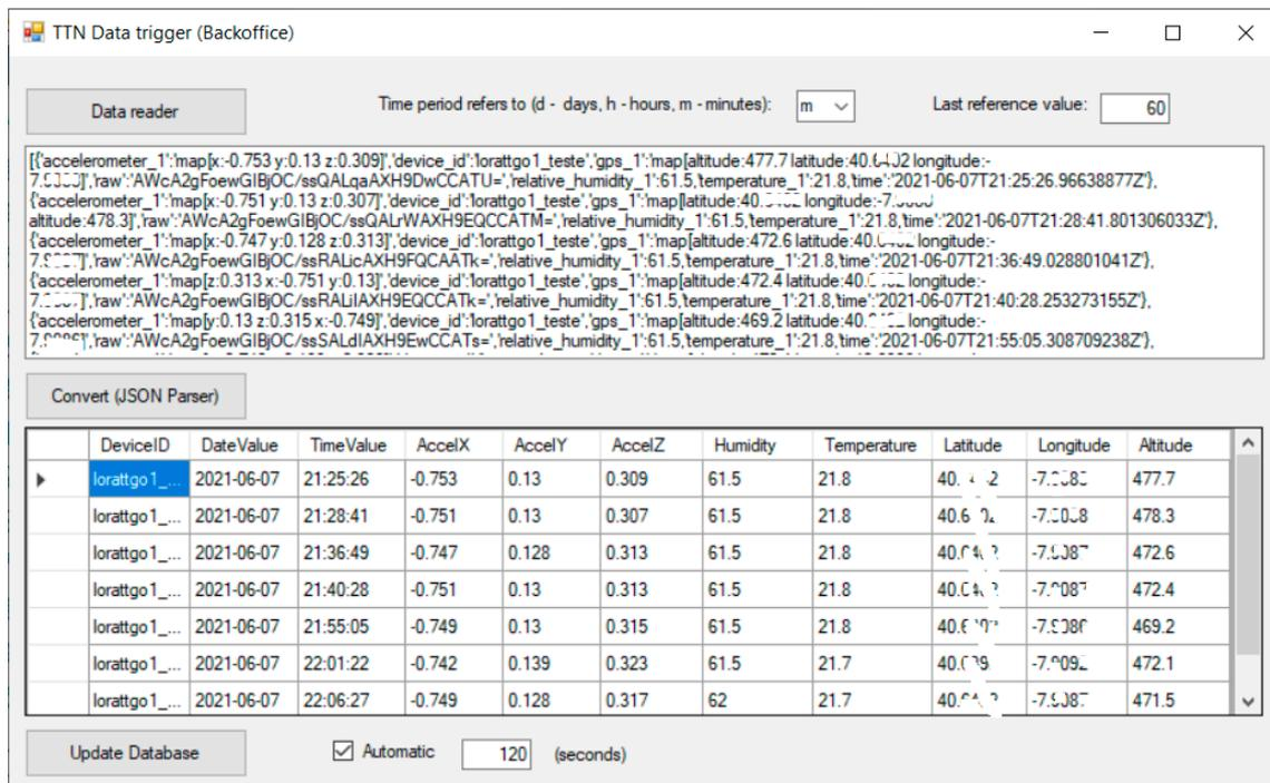
Figure 7. Example of the result obtained in the query from our C# standalone application, in JSON format.
