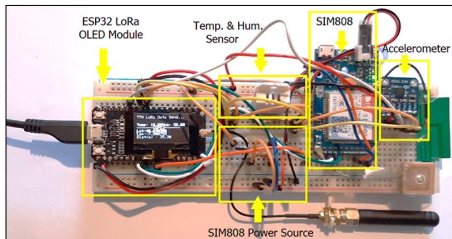
**Figure 6.** Functional prototype in operation powered with USB Power Bank.
