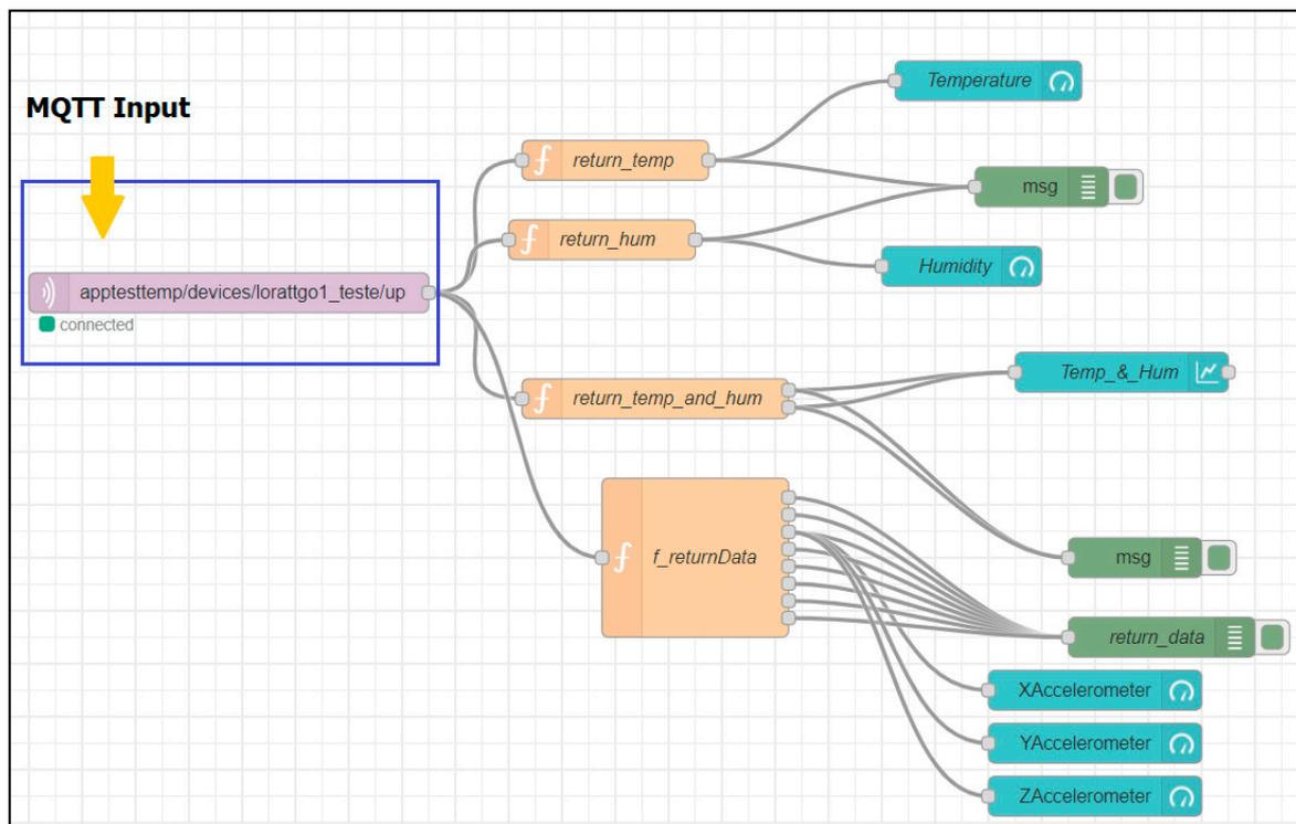
**Figure 1.** Example of MQTT connection to TTN using Node-RED (source: author’s elaboration).
