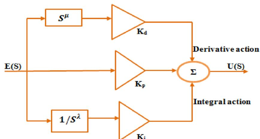
Figure 3. Block diagram of FOPID controller.
