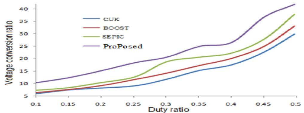
**Figure 11.** Voltage conversion ratio versus duty ratio.
