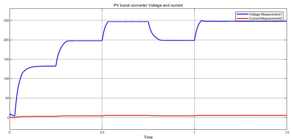
Figure 6. Output voltage/current of the converter.
