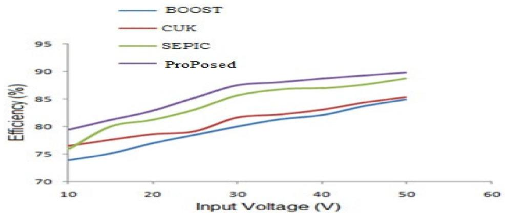
Figure 12. Efficiency versus input voltage.
