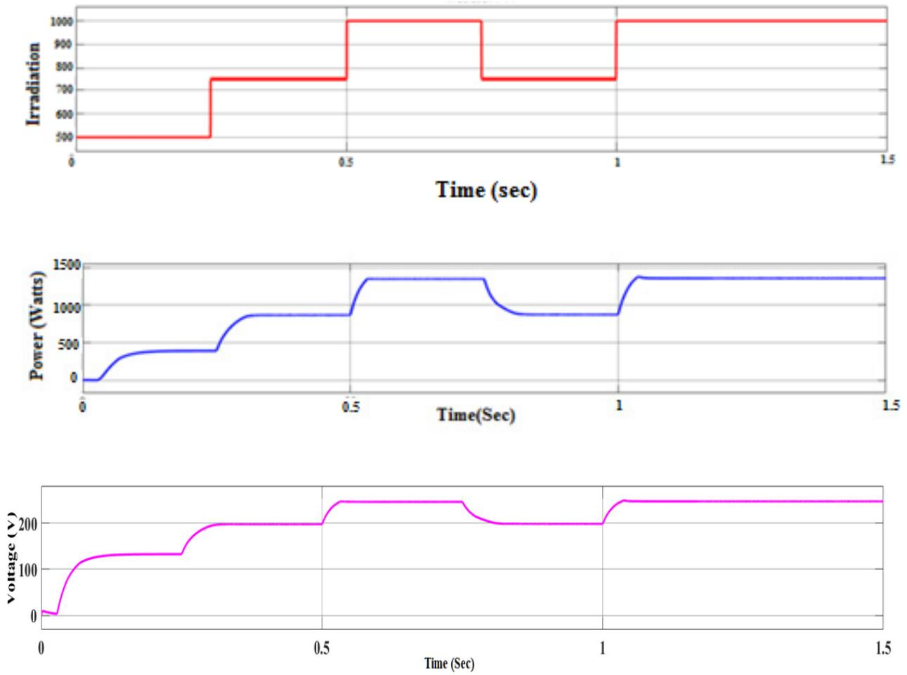
Figure 5. Output PV power and converter voltage with respect to irradiance.
