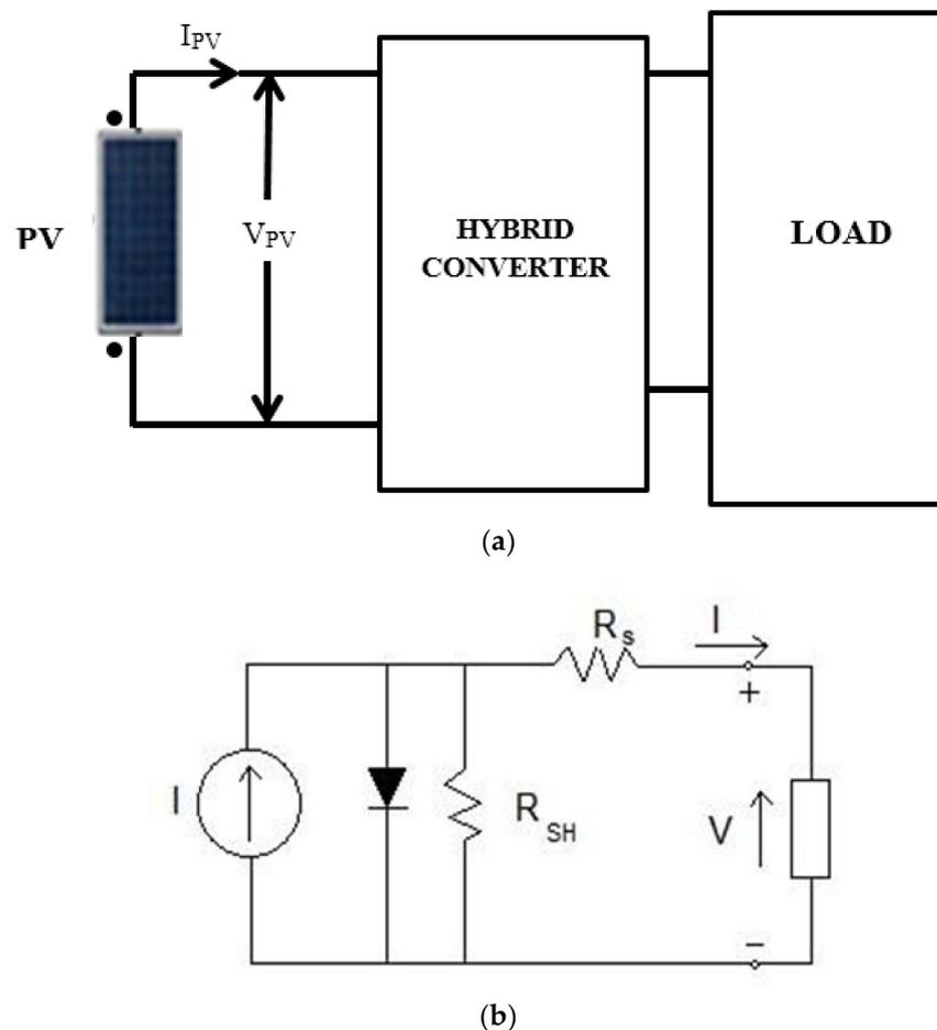
**Figure 1.** (a) Schematic diagram of a proposed module. (b) Diode model of a PV cell.
