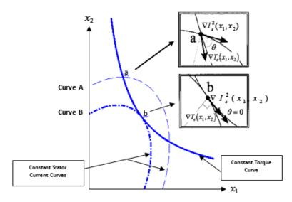
**Figure 3.** The geometric location of the constant torque and the constant stator current in the plane of biaxial currents of torque, adopted from [34].
