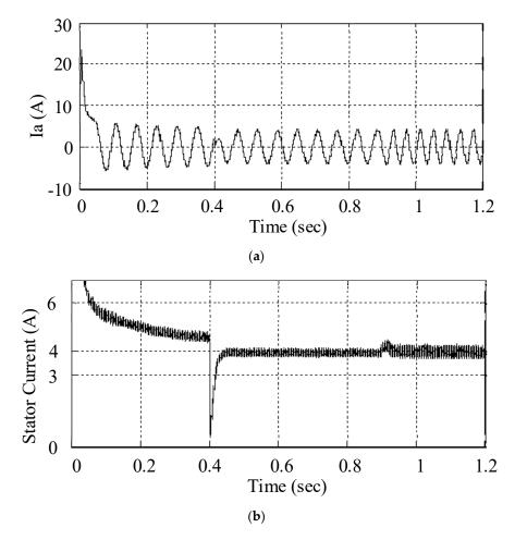
**Figure 12.** Speed and flux control using BELBIC. (a) Stator phase current, (b) current vector of total stator.
