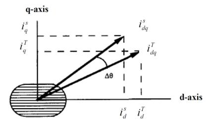
Figure 2. The relationship between torque current and terminal current vector, adopted from [34].
