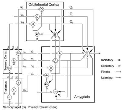
Figure 5. Graphical design of single-layer emotional controller, adopted from [22].
