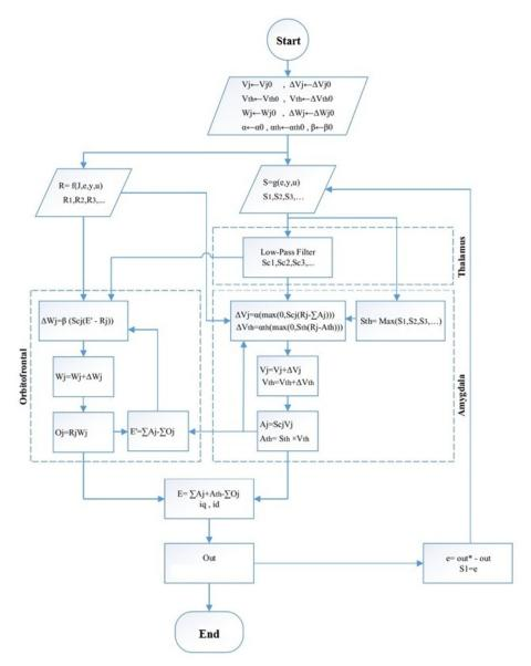
Figure 7. Flowchart and algorithm of emotional control system function.
