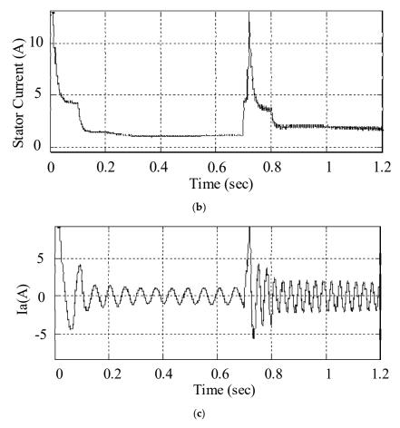
**Figure 14.** Results of optimal control under the MPTA strategy. (a) Magnetic flux, (b) Stator current size, (c) Stator phase current.
