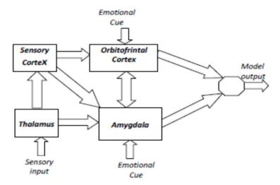
Figure 6. A graphical scheme of the single-layer emotional controller, adopted from [22].
