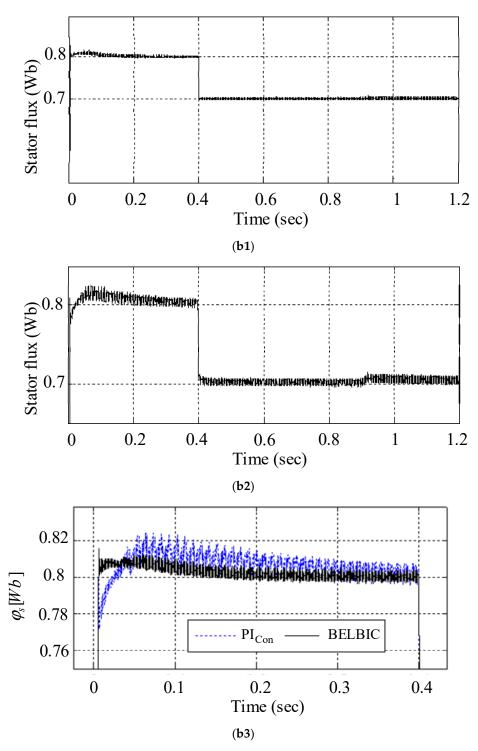
**Figure 11.** Control of velocity and flux using BELBIC and the conventional PI controller regulated by GA. (a) BELBIC electromagnetic torque, (b1) the magnetic flux of the stator, (b2) using the proposed method, (b3) the conventional method [36].
