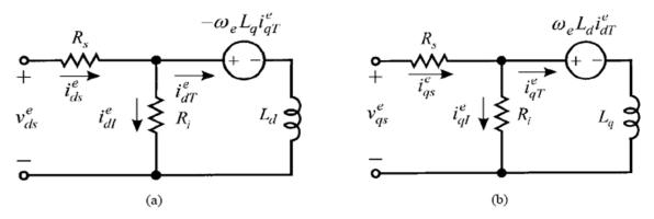
**Figure 1.** Biaxial equivalent circuit of a reluctance synchronous motor by considering iron losses: (a) axis d, (b) axis q adopted from [34].
