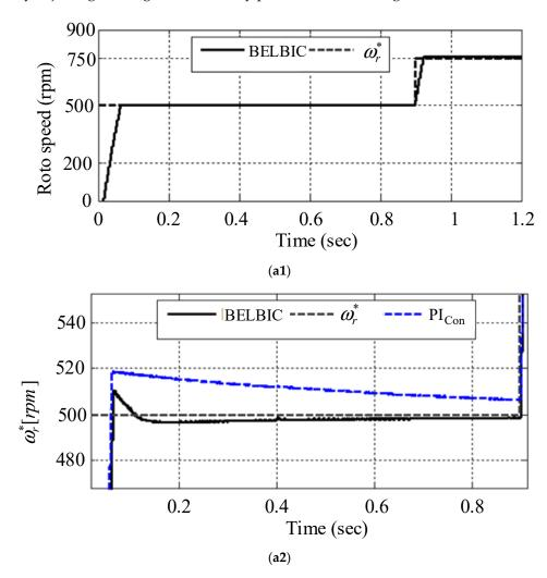
**Figure 10.** Speed and flux control using BELBIC and the conventional PI controller set with GA. (a1) Rotor speed, (a2) Rotor angular velocity.
