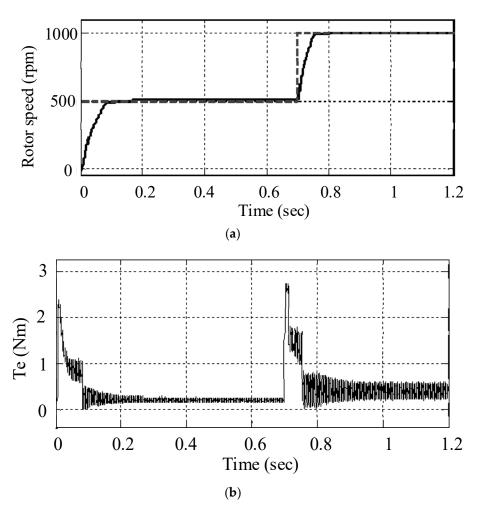
**Figure 13.** Results of optimal control under the MPTA strategy. (a) Rotor speed, (b) electromagnetic torque.
