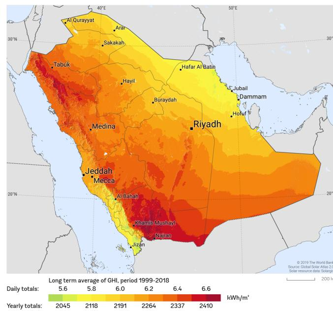
**Figure 1.** Horizontal irradiation showing candidate areas for installing solar PV in Saudi Arabia [12].
