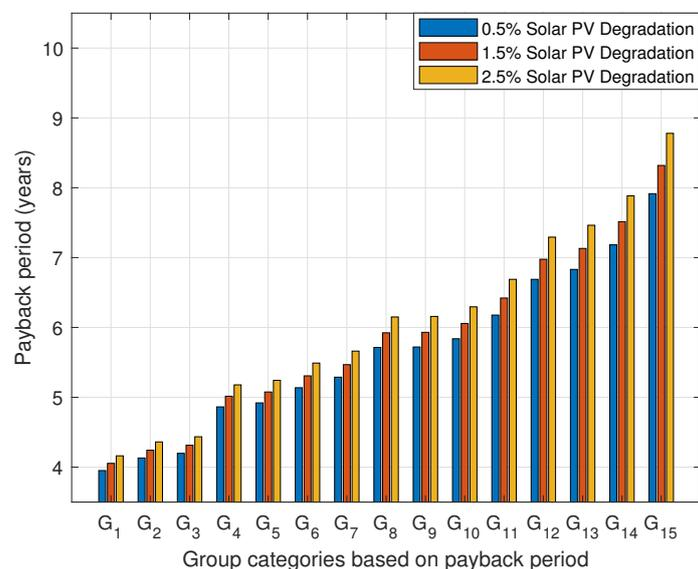
**Figure 8.** Solar PV degradation effect on different categories of payback periods.
