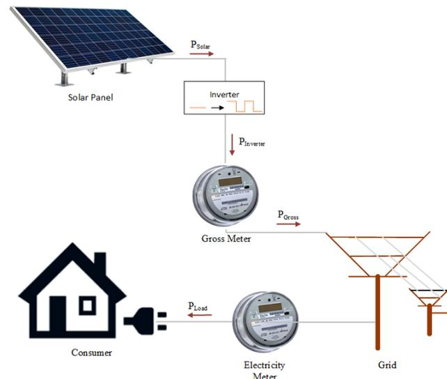
**Figure 3.** Signal flow diagram for gross metering scheme.
