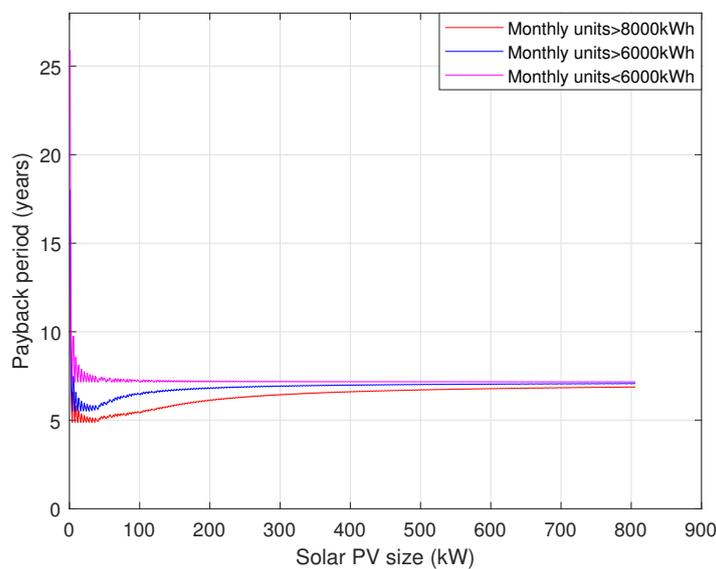
Figure 7. Payback period graph for three commercial loads with maximum area.
