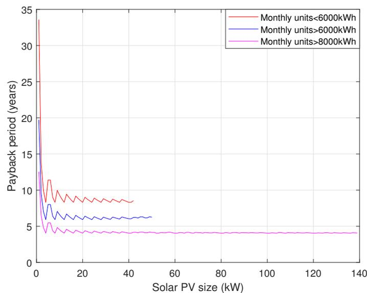
**Figure 4.** Payback period behaviour against solar PV size for three different residential loads with limited area.
