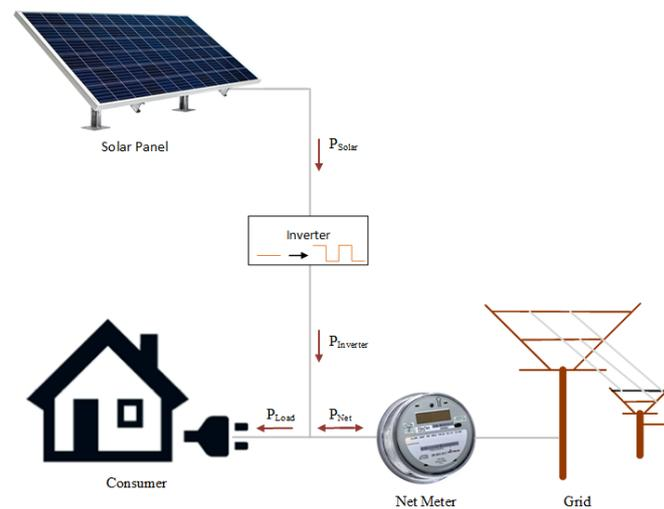
**Figure 2.** Signal flow diagram for net metering scheme.
