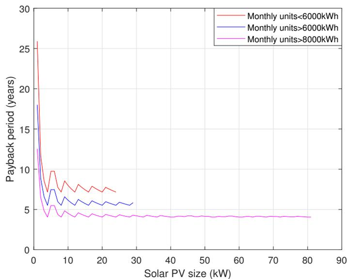
Figure 6. Payback period curves for three different commercial loads with limited area.
