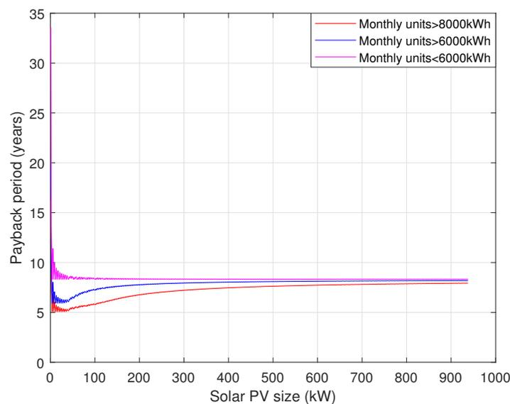
**Figure 5.** Payback period trends for three different residential loads with maximum area.
