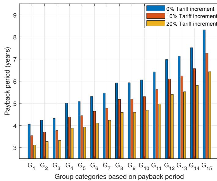
Figure 9. Effect of SEC tariff increment per kilowatt hour on different categories of payback periods.
