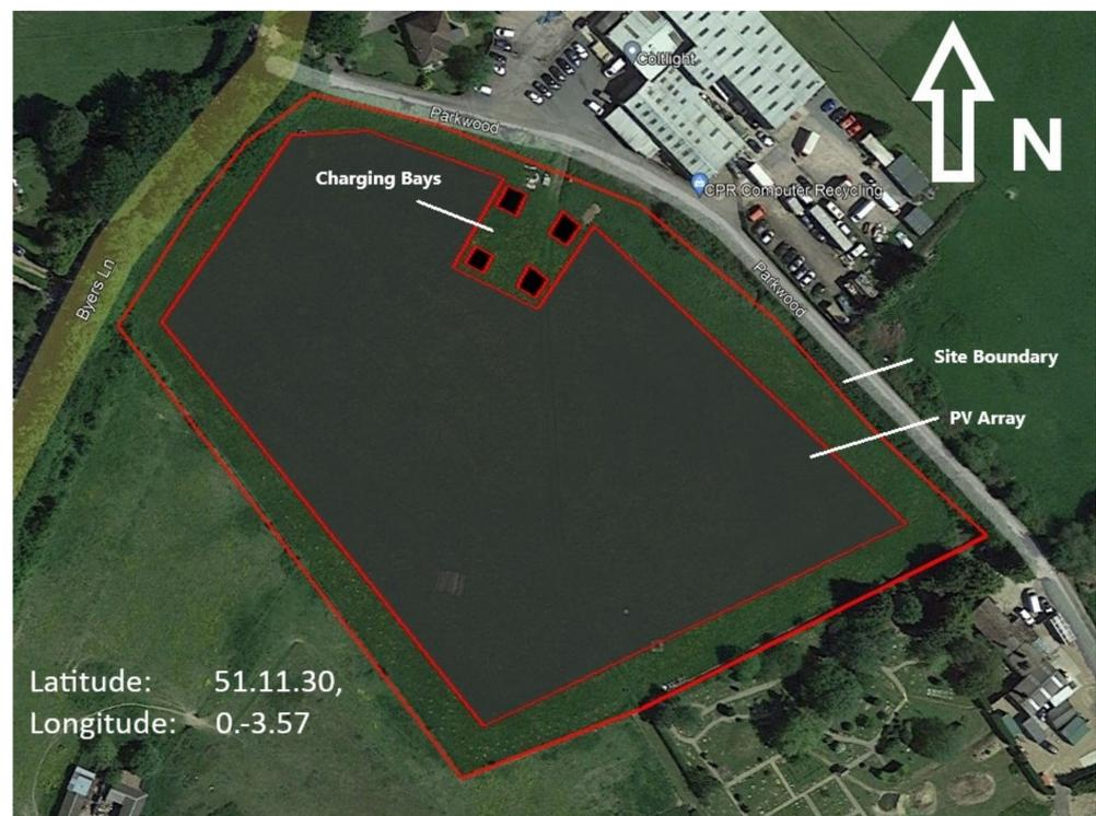
**Figure 2.** The PVEVCS layout and site diagram, as seen using Google Earth Pro.
