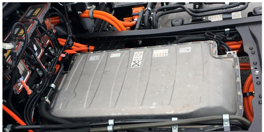
**Figure 16.** Chassis layout of a Mitsubishi Fuso E-canter, highlighting a sealed battery pack and organised orange HV cabling. Photo taken by the author.
