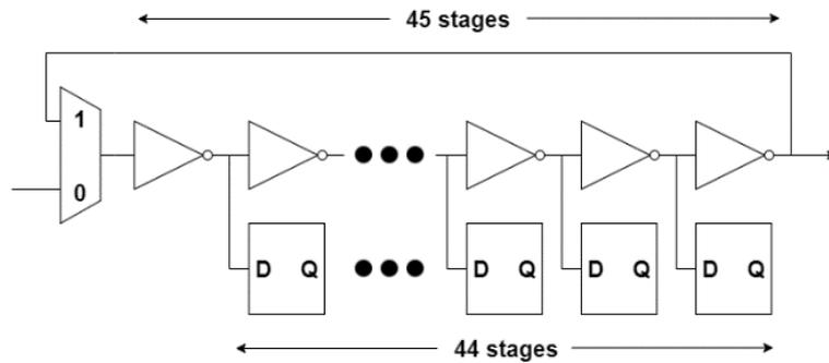
Figure 9. Schematic of the 28-nm RO design.
