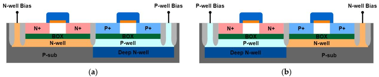
Figure 4. (a) Flipped well configuration (FBB); (b) regular well configuration (RBB).
