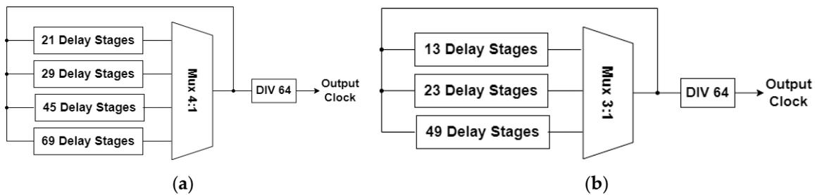
**Figure 2.** Schematic designs of different gate-based ROs: (a) Inverter-based RO schematic design; (b) NAND2 or NOR2-gate-based RO schematic design.
