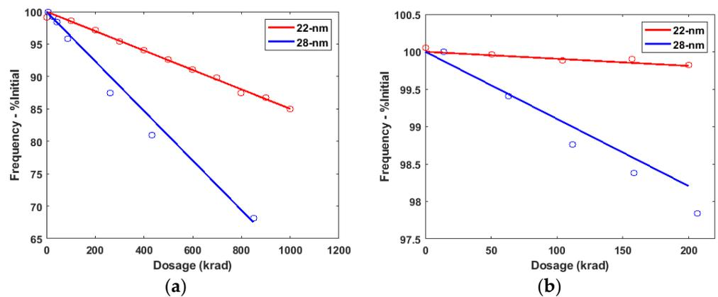
Figure 10. RO frequencies from 22-nm and 28-nm test for (a) Co-60 test; (b) heavy ion test.
