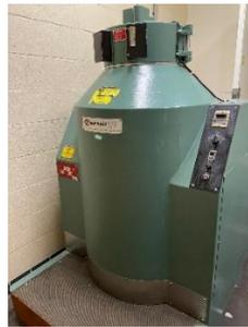
Figure 6. Gammacell 220 Co-60 Irradiator.
