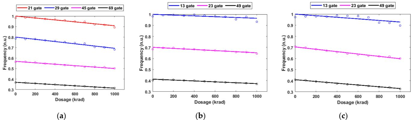
Figure 7. RO frequencies vs. total absorbed dose during Co-60 test: (a) Inverter-based ROs; (b) NAND2-based ROs; (c) NOR2-based ROs.
