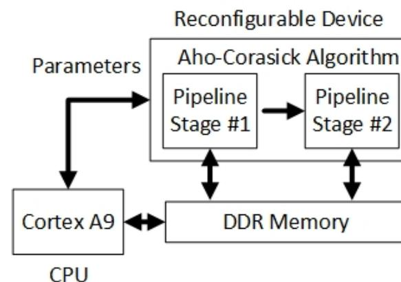
**Figure 4.** Reconfigurable Aho–Corasick architecture.
