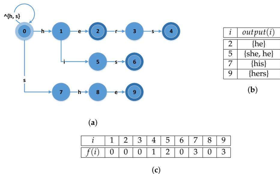
**Figure 2.** An example of multi-pattern matching with Aho–Corasick. (a) The Aho–Corasick goto function, presented as a state machine for the patterns she, he, hers, his. (b) The output function, indicating the final state of each pattern in the given set. (c) The Aho–Corasick failure function for the given pattern set.
