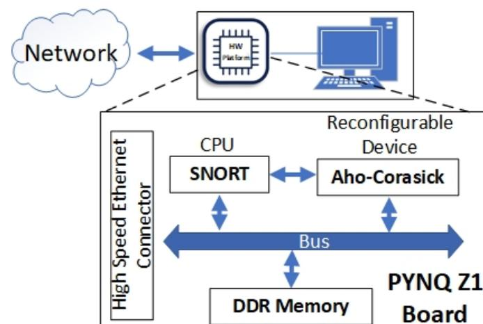
**Figure 5.** Reconfigurable Aho–Corasick architecture is integrated with the official Snort IDS on a PYNQ Z1 board.
