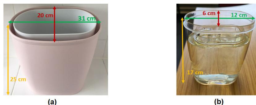
**Figure 1.** (a) Fabricated realistic torso phantom used for measurements inside anechoic chamber; (b) the miniaturized torso phantom (here without inclusion) used for MammoWave device's measurements.
