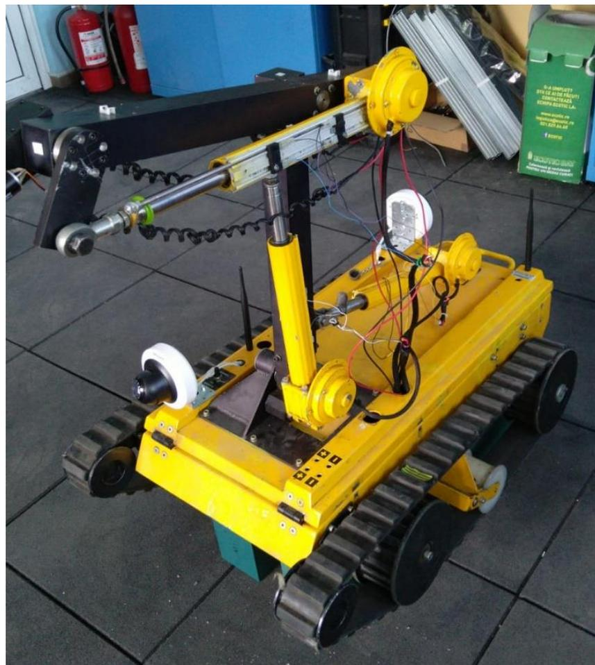
**Figure 1.** The analyzed EOD robot.
