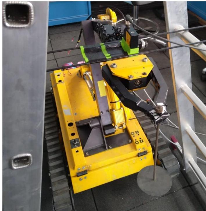
**Figure 2.** The analyzed EOD robot and the hook for positioning the working weights.
