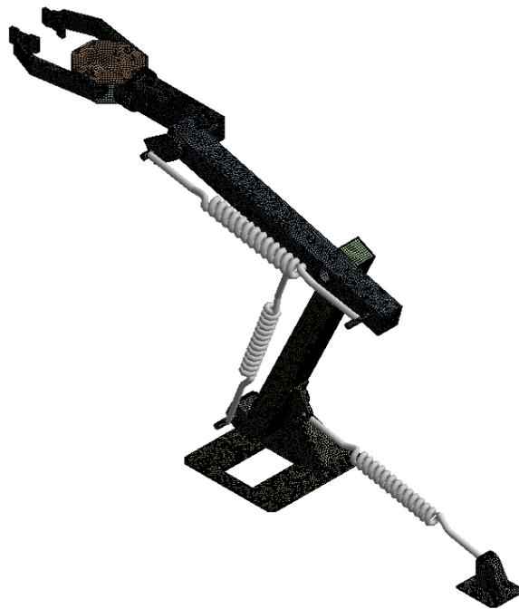
**Figure 13.** Representation of the finite element model in which the linear motors are replaced by elastic elements.
