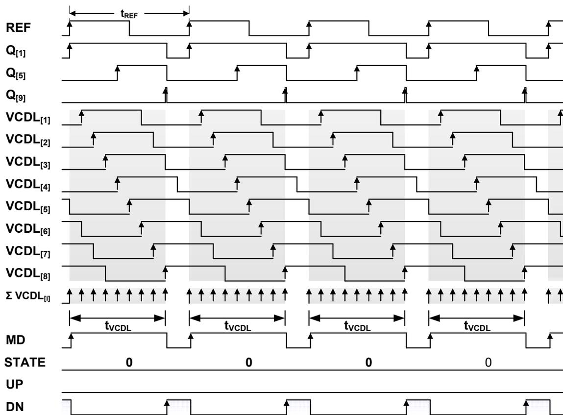
Figure 5. Timing diagram for the PD-MDV operation under the condition  $t_{VCDL} < t_{REF}$ .
