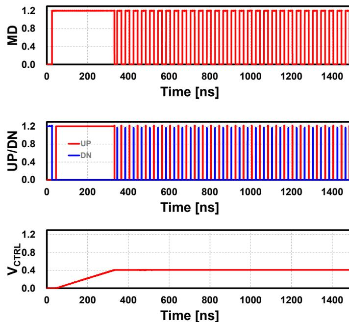
**Figure 10.** The locking behavior of the PD-MDV according to a 0 V  $V_{CTRL}$  initial condition at  $f_{REF} = 50$  MHz.
