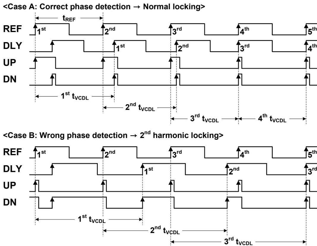
**Figure 2.** Two different operations of conventional PD under the same input condition as  $1^{\text{st}} t_{\text{VCDL}} > t_{\text{REF}}$  (Case A: Correct phase detection; Case B: Wrong phase detection).
