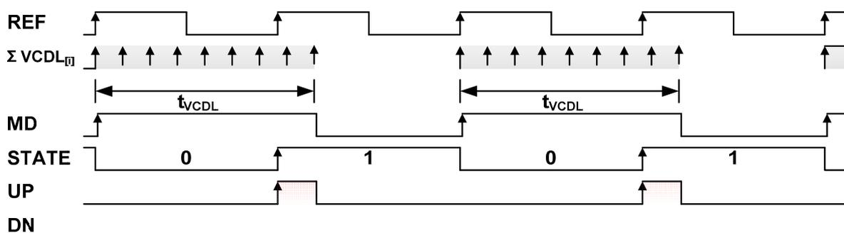
Figure 6. Timing diagram for the PD-MDV operation under the condition  $t_{REF} < t_{VCDL} \leq 2 \cdot t_{REF}$ .
