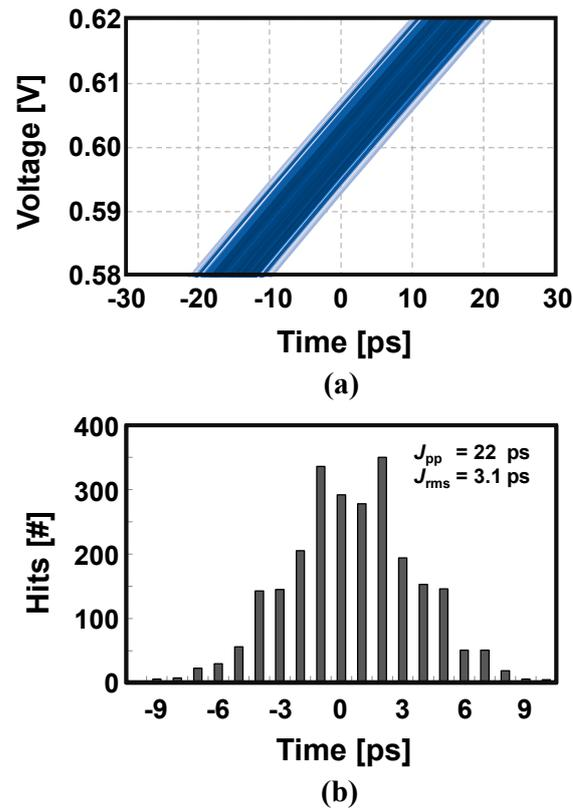
**Figure 11.** Jitter simulation at 200 MHz: (a) overlapped waveforms of 256 cycles; (b) histogram of 2500 samples.
