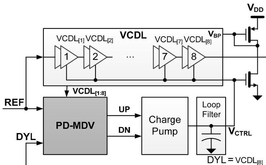
Figure 3. The structure of the proposed PD-MDV DLL.
