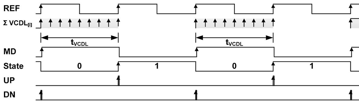
Figure 8. Timing diagram under condition of DLL locking with PD-MDV.
