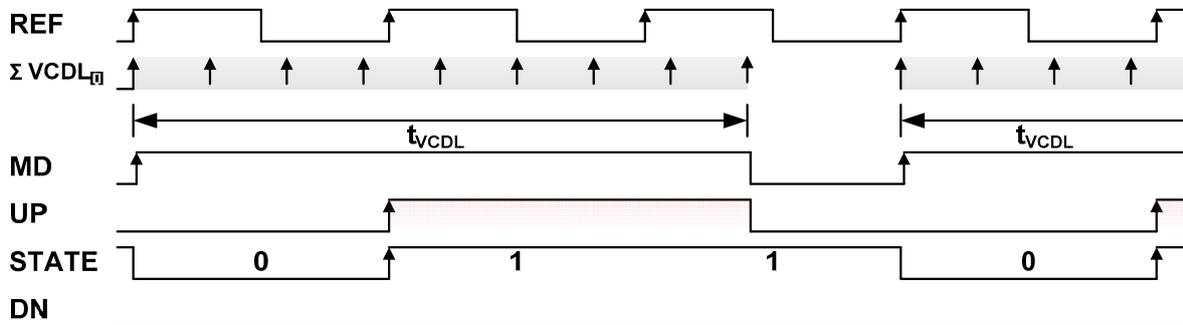
Figure 7. Timing diagram for the PD-MDV operation under the condition  $t_{VCDL} > 2 \cdot t_{REF}$ .
