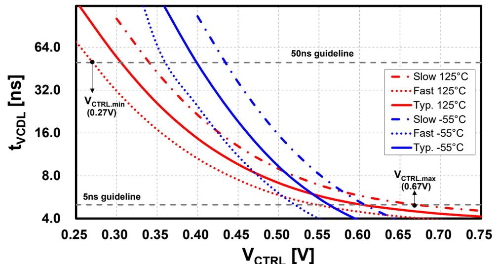
Figure 9. Characteristics of the delay of the VCDL according to  $V_{CTRL}$ , temperature, and process corner to design the output swing range of charge pump.
