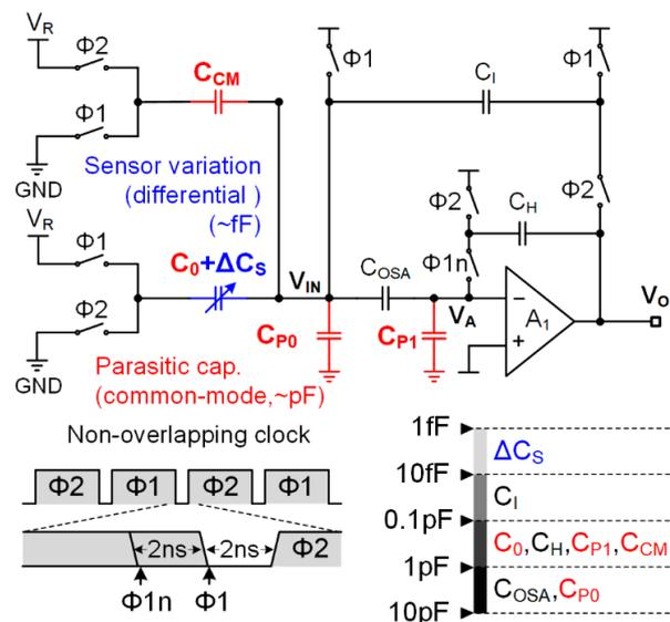
Figure 2. Schematic, timing diagram, and typical capacitance value of traditional switched-capacitor capacitance-to-voltage converter (SC-CVC) of readout circuit.
