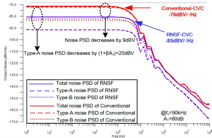
Figure 12. The PSD of RNSF-CVC and conventional CVC.
