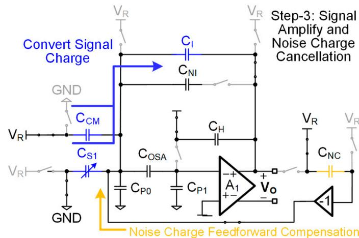
Figure 8. The signal amplification and noise charge cancellation phase of reset noise sampling feedforward technique.
