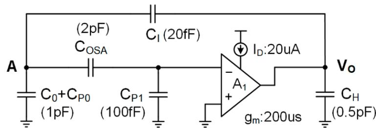
**Figure 10.** Equivalent circuit model with typical component parameters of CVC during signal amplification phase ( $\Phi 2$  for conventional SC-CVC &  $\Phi 3$  for RNSF-CVC).
