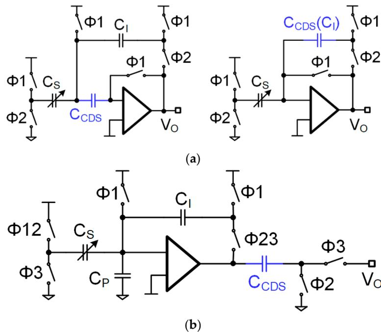
Figure 9. Summary of the CDS technique. (a) Type-I (left) and Type-II (right). (b) Type-III.
