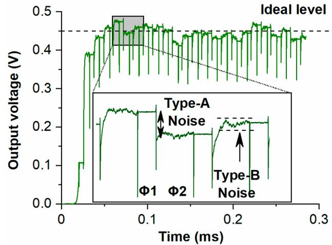
Figure 3. The typical transient output noise waveform of CVC.
