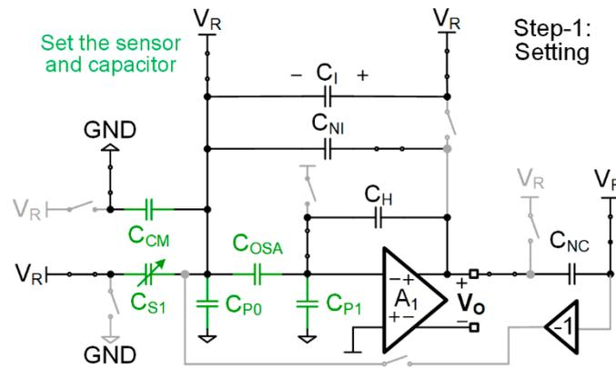
Figure 6. The setting phase of the reset noise sampling feedforward technique.
