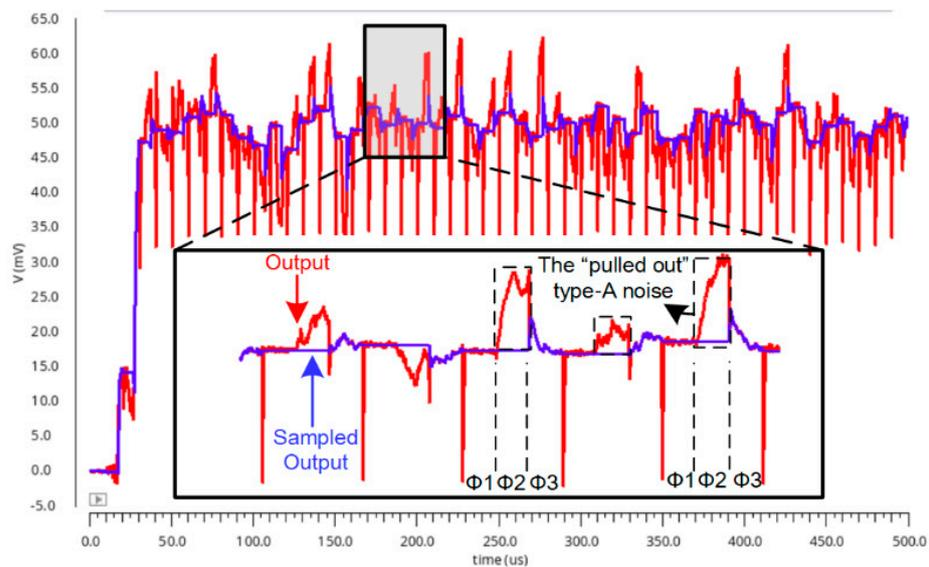
**Figure 11.** The transient output waveform of RNSF-CVC.
