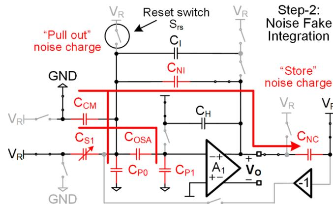
Figure 7. The noise fake integration of the reset noise sampling feedforward technique.
