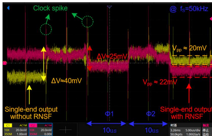
Figure 16. The measurement transient waveform of the output noise of the readout circuit with the RNSF technique and without the RNSF technique.
