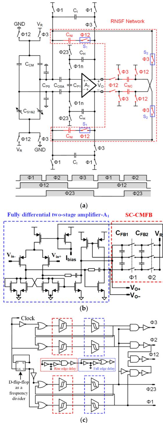
**Figure 5.** Circuit implementation of proposed capacitance-to-voltage converter based on the RNSF technique for a differential MEMS capacitive accelerometer. (a) Schematic and timing diagram. (b) Fully differential two-stage amplifier with SC-CMFB. (c) Three-phase non-overlapping clock generator.
