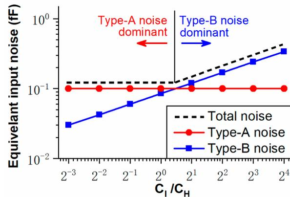
Figure 4. The relationship of type-A equivalent input noise, type-B equivalent input noise and ratio  $C_I/C_H$ .
