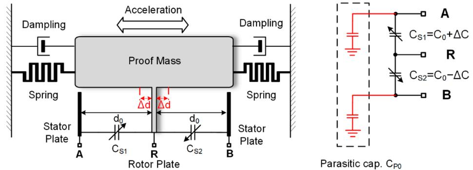
Figure 1. Sensing element of a typical MEMS capacitive accelerometer.
