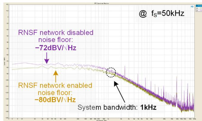
**Figure 17.** Measurement results of the output PSD of readout circuit with the RNSF technique and without the RNSF technique.
