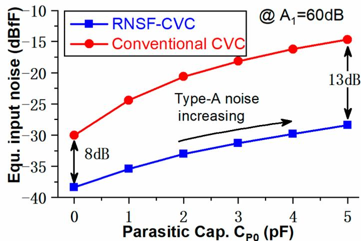
Figure 13. The noise reduction effectiveness of the RNSF technique varies with parasitic capacitance.
