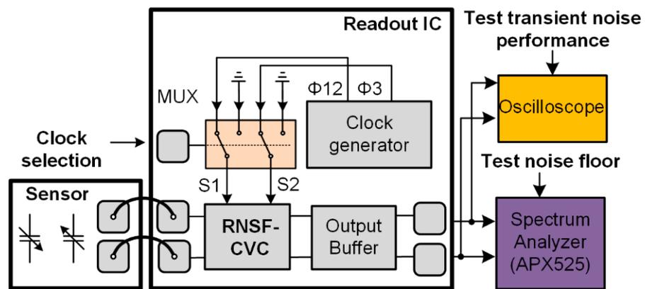
Figure 15. The test configuration of the readout IC.
