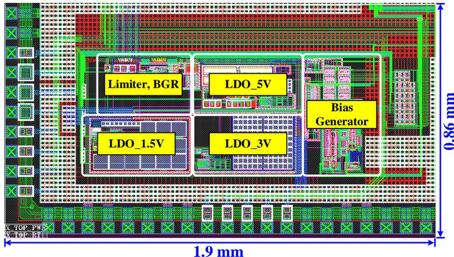
Figure 5. Top layout pattern of the proposed power regulated circuit (PRC).
