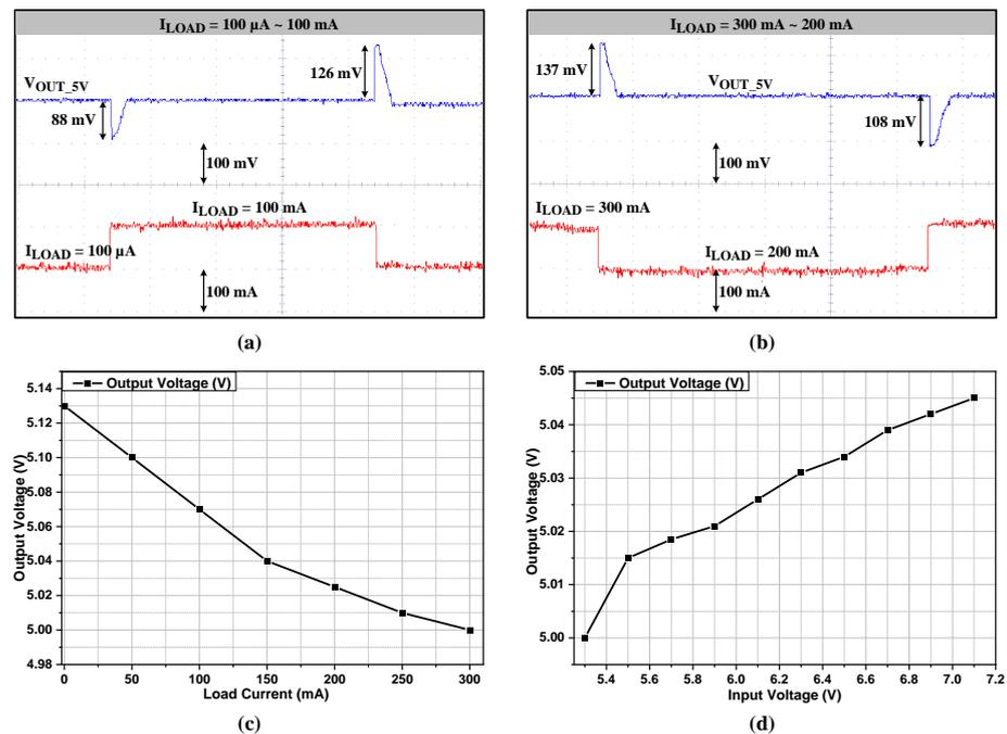
Figure 8. Measured results of LDO\_5V. (a) Load transient response from 100  $\mu$ A to 100 mA. (b) Load transient response from 300 mA to 200 mA. (c) Load regulation. (d) Line regulation.
