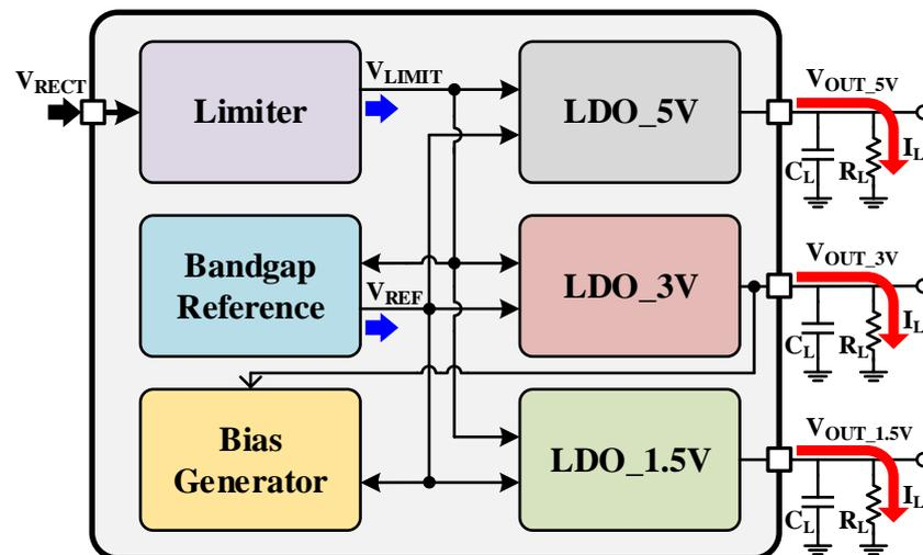
Figure 1. Block diagram of the proposed power regulated circuit (PRC).
