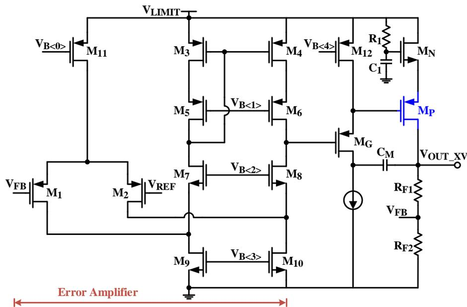
Figure 4. Circuit diagram of the proposed low-dropout regulator (LDO) in the PRC.
