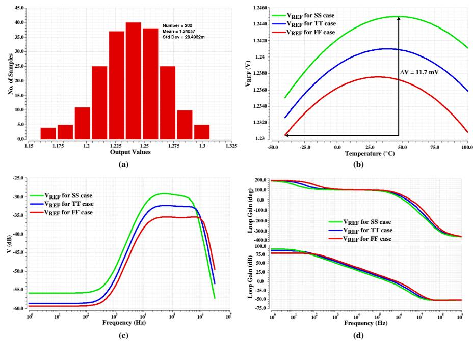
Figure 7. Post-simulation results of the proposed BGR. (a) Monte Carlo simulation. (b) Output voltage’s variation over temperature range. (c) PSRR for different corner cases. (d) Stability check.
