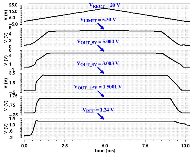
Figure 6. Top simulation results of the proposed power regulated circuit (PRC).
