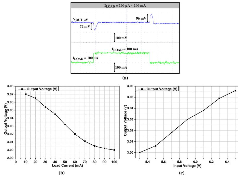
Figure 9. Measured results of LDO\_3V. (a) Load transient response from  $100\ \mu\text{A}$  to  $100\ \text{mA}$ . (b) Load regulation. (c) Line regulation.
