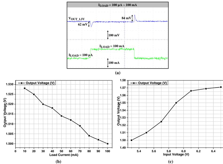
Figure 10. Measured results of LDO\_1.5V. (a) Load transient response from  $100\ \mu\text{A}$  to  $100\ \text{mA}$ . (b) Load regulation. (c) Line regulation.
