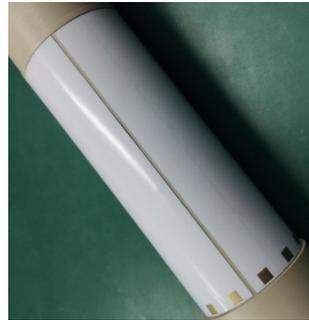
**Figure 1.** ECT sensor machined with FPC electrode process and cut PEEK pipe process.
