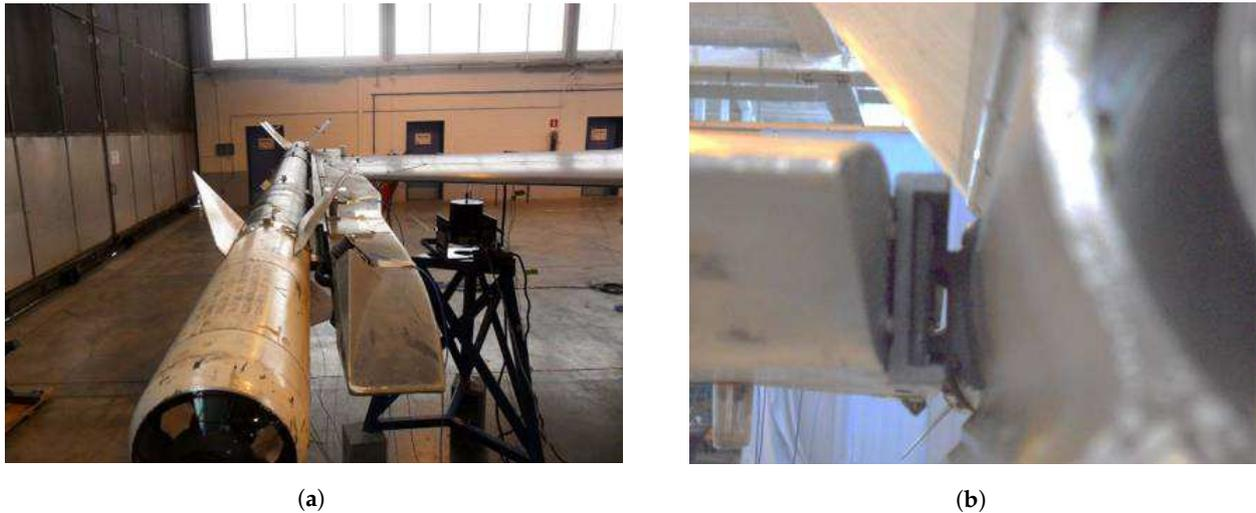
**Figure 2.** (a) Dummy payload mounted at the right wing tip. (b) Connection of the right-wing-to-payload mounting interface. Reproduced under CC BY-SA 4.0 from [46].
