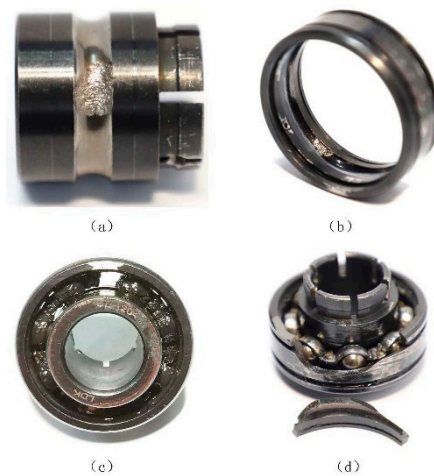
Figure 9. Bearing pictures of typical failure types. (a): Inner race wear (b): Outer race wear (c): Cage fracture (d): Outer race fracture.
