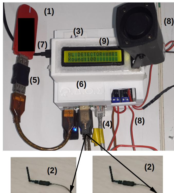
**Figure 3.** BL-detector end node device prototype and detector enumerated hardware parts.
