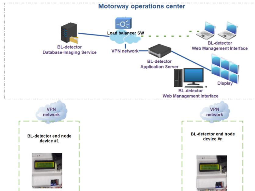
Figure 1. BL-detection system high-level architecture.
